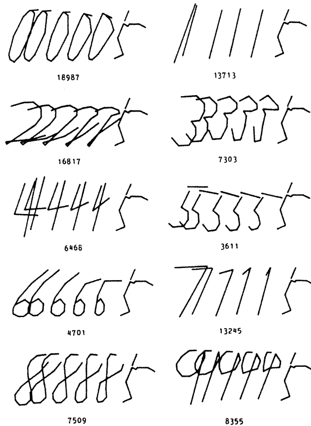
Fig. 4. Example showing the recognition process for one unknown numeral. Each of the reference shapes (left) is stretched onto the unknown shape (right), and the template match is computed (bottom). The number is recognized correctly as a "five" since the reference five produced the best template match. Notice the tolerance to segmentation irregularity and spurious lines.
