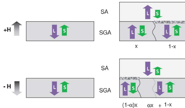
Figure 12: Sketches of the magnetic configuration below the SGA compensation temperature in the single SGA layer (left) and in the SGA/SA bilayer (right) for positive (top) and negative (bottom) fields. In the SGA/SA bilayer, x corresponds to the proportion of L-up domains for the positive field, \alpha x is the proportion of L-up domains that reverses toward L-down for the negative field (from [17] ).
