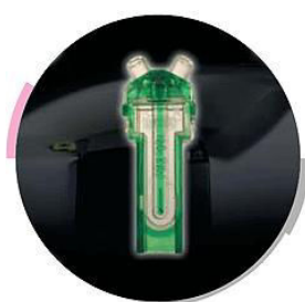
Figure 120. The capillary zeta potential cell for the Malvern Zetasizer.
