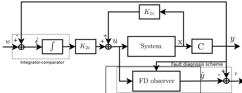
Figure C.1 – Fault diagnosis and Tracking controller scheme
