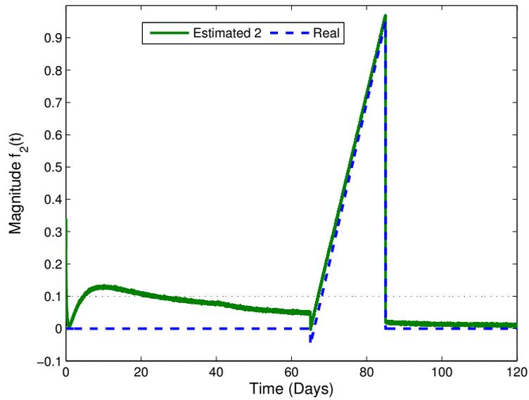
Figure 3.14 – Fault 2 and its estimation.
