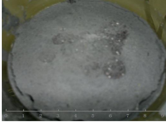
Figure 3. 14: Appearance of the ashes after filtration (the white spots are \text{CaCO}_3 )
