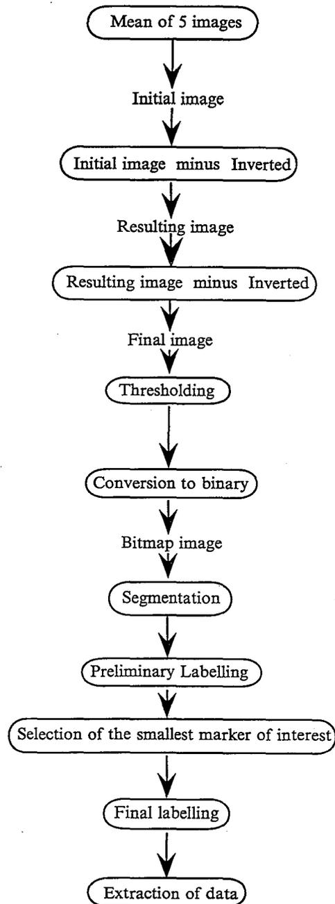
FIG. 2. Image processing algorithm.
