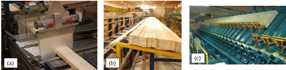
Figure 2.19 – (a) application de colle, (b) assemblage des lamelles, (c) pressage.
