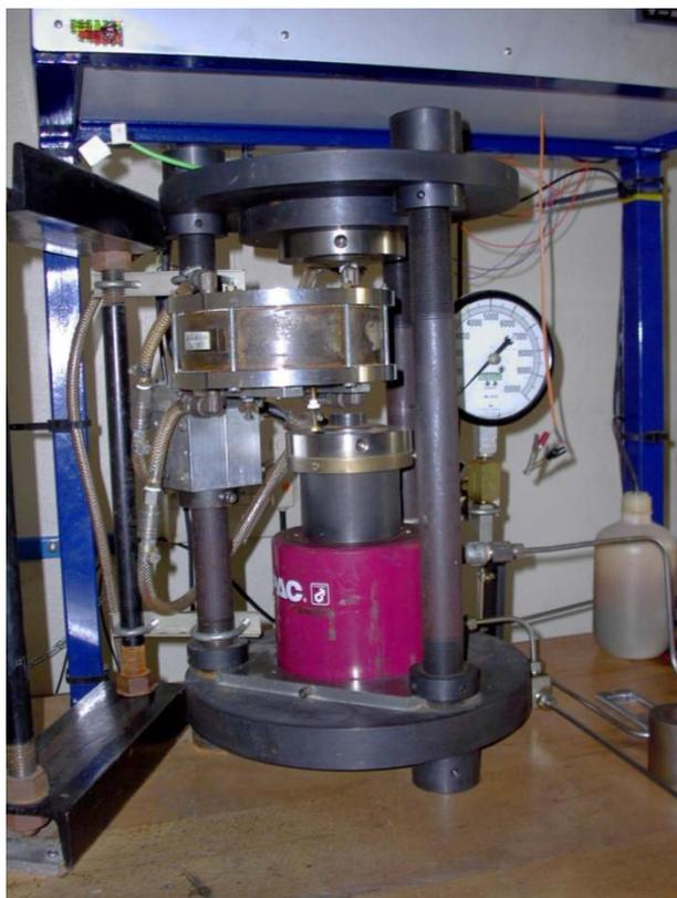
*Figure 2.5: Piston-cylindre sans contre-pression
