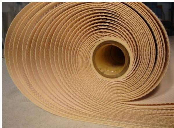
Figure I-13. Module spiralé (source : [www.cmtmembrane.com](http://www.cmtmembrane.com))
