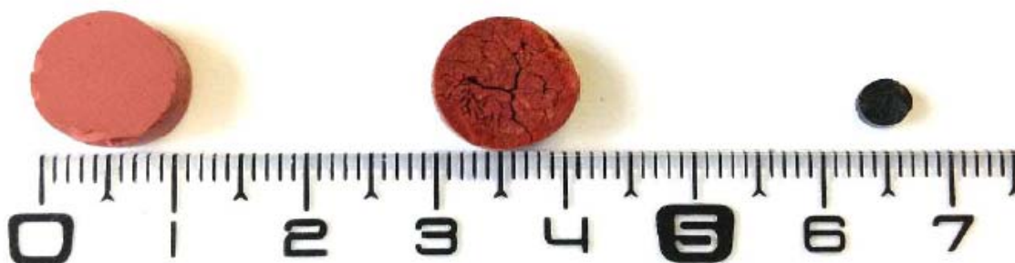
Fig. 79: The three dried gels made from tannin and formaldehyde resin and dried in supercritical CO 2 conditions (aerogel) on the left; freeze-drying conditions (cryogel) on the centre and subcritical conditions (xerogel) on the right.
