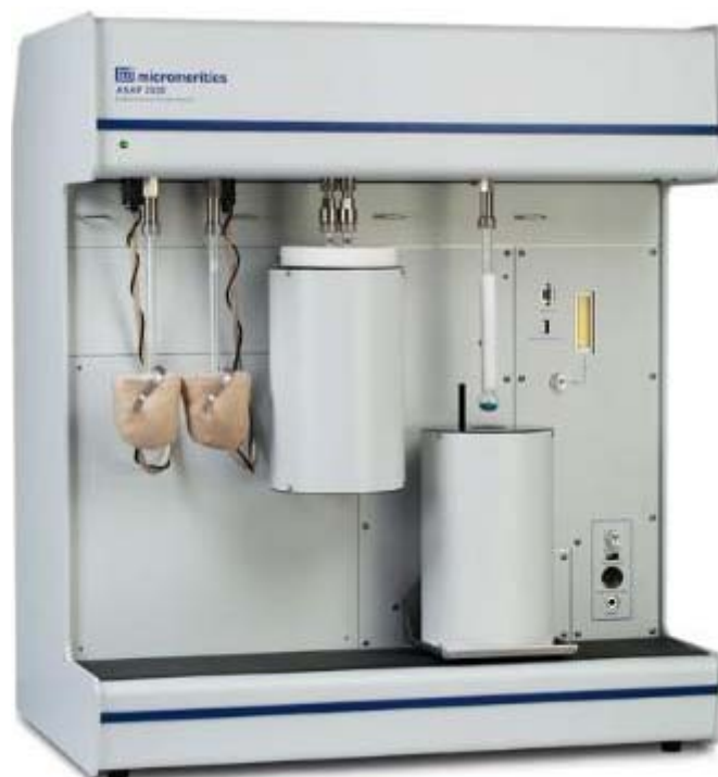
Fig. A5: Micromeritics ASAP 2020 instrument used for the adsorption-desorption experiments.
