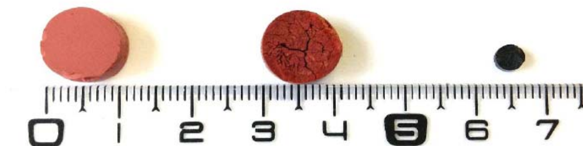
Fig. 79: The three dried gels made from tannin and formaldehyde resin and dried in supercritical CO 2 conditions (aerogel) on the left; freeze-drying conditions (cryogel) on the centre and subcritical conditions (xerogel) on the right.
