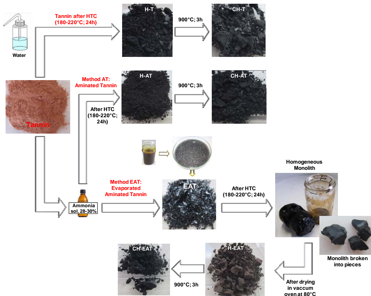
Fig. 60: The methods used for preparing N-doped carbon materials and their respective final products.
