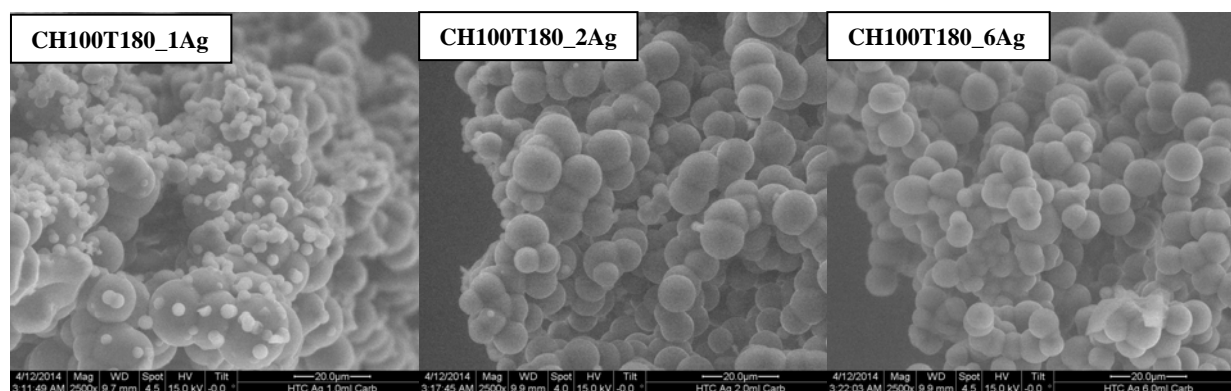
Fig. 56: TEM images of three filtrates obtained after HTC of tannin with 1, 2 or 6 mL of 0.1M AgNO_3 solution at 180°C for 24h and posterior carbonization at 900°C.
