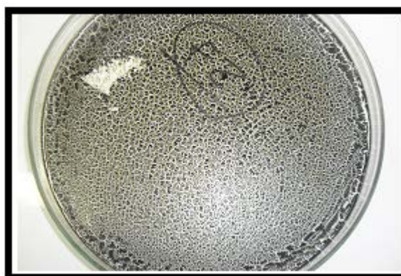
Figure 1. Appearance of a gelled aminated tannin (FZ formulation, Table 1) showing the granular nature and absence of film forming.
