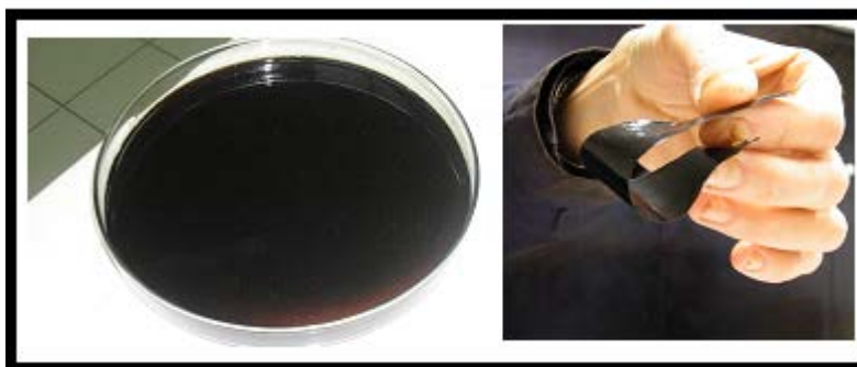
Figure 2. Appearance of a flexible film formed onto a glass support and of its level of flexibility for a formulation of aminated tannin reacted with furfuryl alcohol – F12 formulation).
