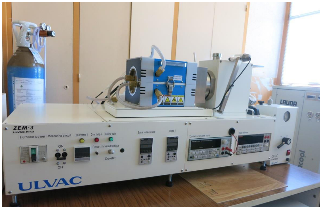
Figure IV-11: Photography of the ZEM-3 measurement system.
