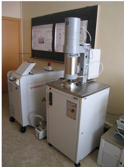
Figure IV-8: Photography of the thermal diffusivity measurement system (LFA 427, Netzsch).
