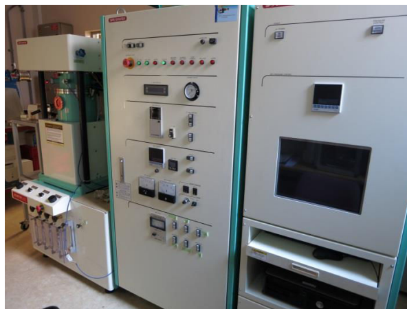
Figure III-9: Dr Sinter 515S SPS Syntex Inc. installed at IJL.
