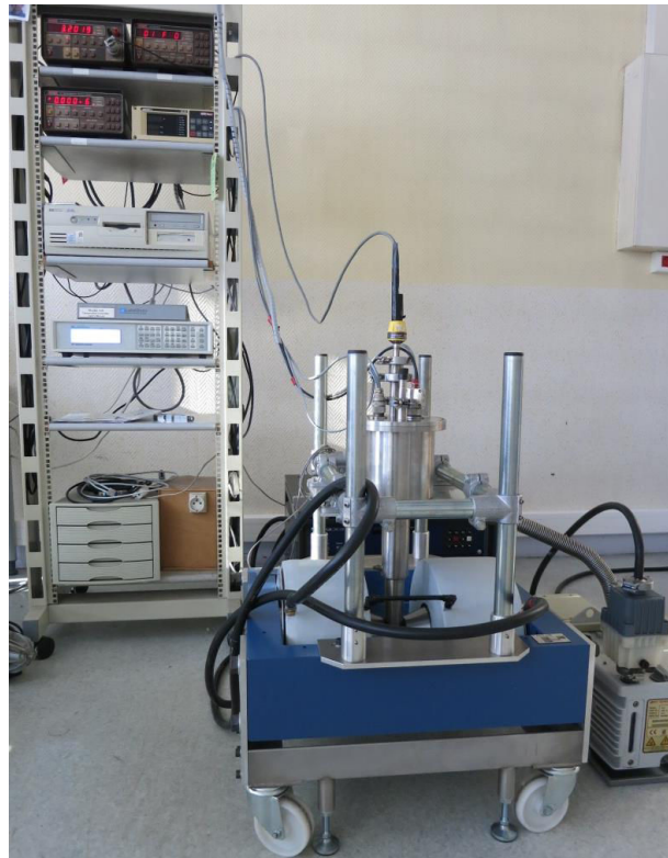
Figure IV-13: High temperature galvanomagnetic properties measurement system.
