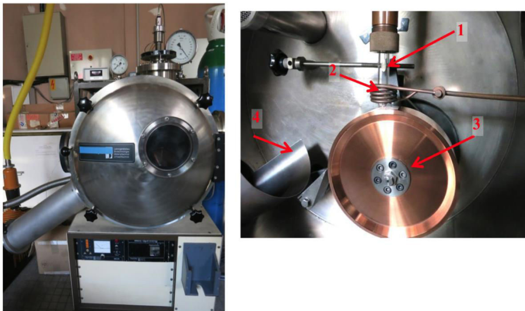
Figure III-5: Edmund Bühler melt-spinner located in IJL. Left: general view; right: inner chamber design, where 1 – crucible, 2 – induction coil, 3 – copper wheel, 4 – material collector.
