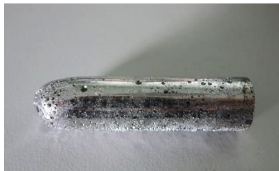
Figure III-2: Image of the initial ingot obtained after quenching in water (WQ in table III-1).
