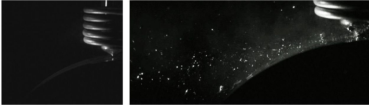
Figure III-7: Images taken by a high-speed camera before the melt ejection (left) and during the melt-spinning process (right).
