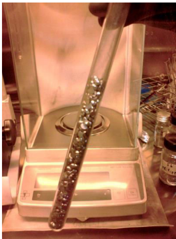
Figure III-1: A quartz tube with the total amount of pure elements (about 50 g) inside the glove box.
