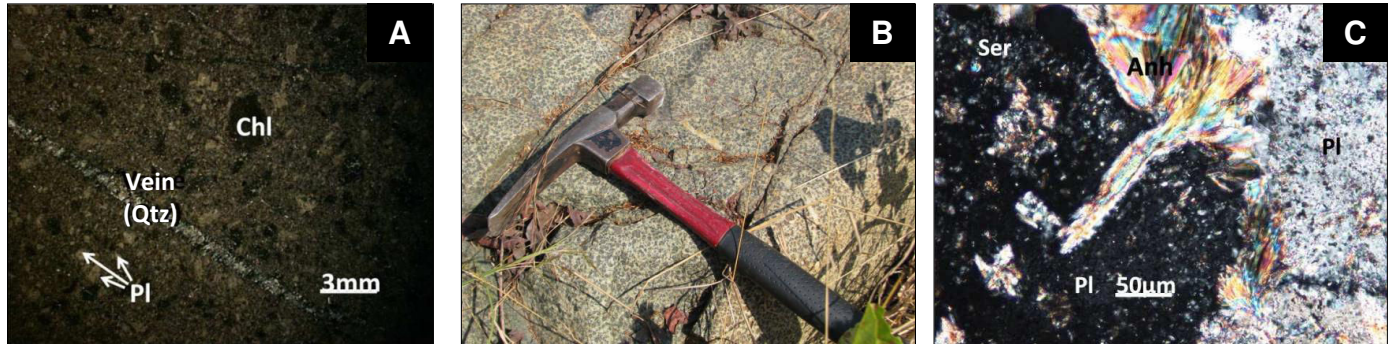
Figure 3: Macro- and microphotographs of the volcanic and plutonic host rocks of Gaoua occurrences. A: Volcanic facies expressing strong chloritisation (Chl) crosscut by quartz (Qtz) veins. B: Gabbroic plutonic facies. C: Dioritic plutonic facies, with plagioclase (Pl) surrounding anhydrite (Anh) and showing sericitization (Ser).
