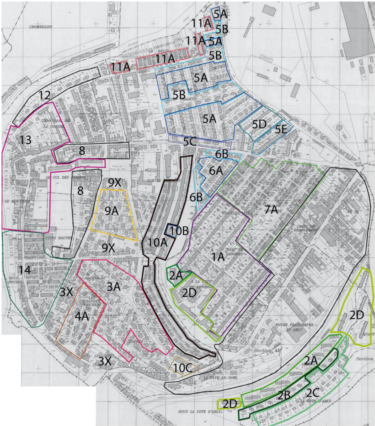
Figure 70. Map of Joazeuf city with the zones according to the construction eras, the geometrical characteristics, and the structural properties of the buildings
