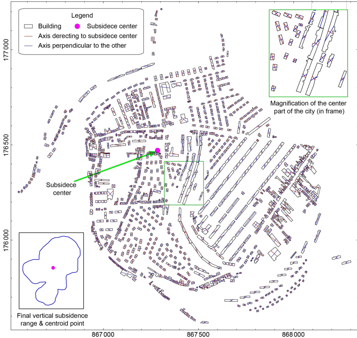
Figure 74. Selection of the axes where the structural models will be performed for each building: using the axis from the building centroid point directing to the subsidence center and the axis perpendicular to the former at the building centroid (not suitable and rejected)
