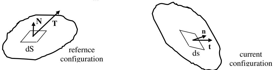
Fig. C.2.2 Traction vectors \mathbf{T}, \mathbf{t} in undeformed and deformed configurations respectively
