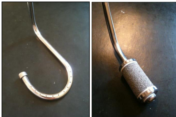
Figure 41. Picture of the classic sparger 1000μm (left) and the microsparger, two porosities: 20μm and 40μm (right)
