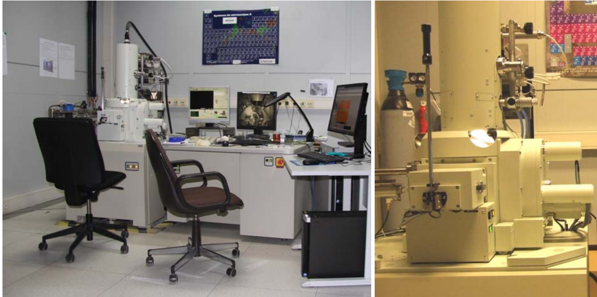
Figure 57 – Field Emission Gun Scanning Electron Microscope (FEG SEM) JEOL 7001F.
