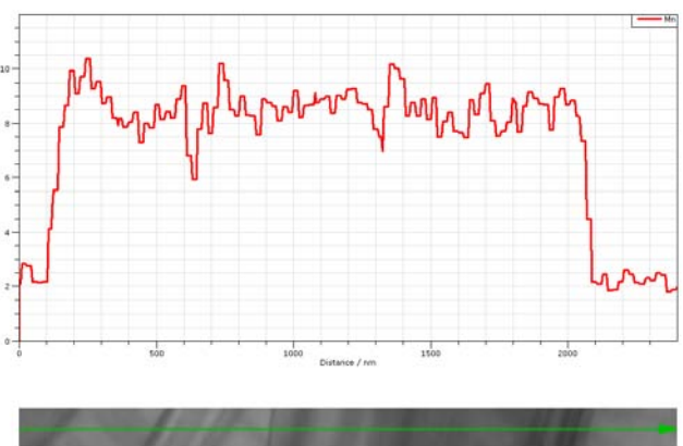
Figure 175 – Mn profiles of 10h sample: at left are presented selected zones and at right – corresponding Mn evolutions as a function of distance.
