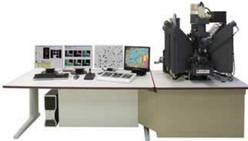
Figure 61 – CAMECA SX100 Electron probe microanalyzer.
