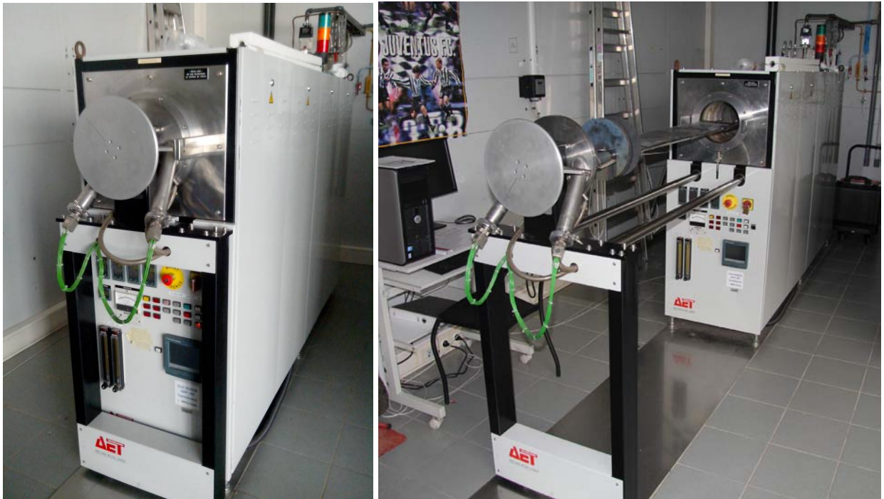
Figure 46 – AET Gradient Batch Annealing (GBA) furnace.
