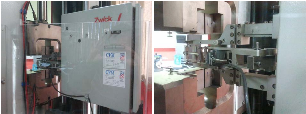
Figure 51 – MacroXtens SE50 extensometer: at left – global view; at right – zoom on the part which is in contact with tensile specimen.
