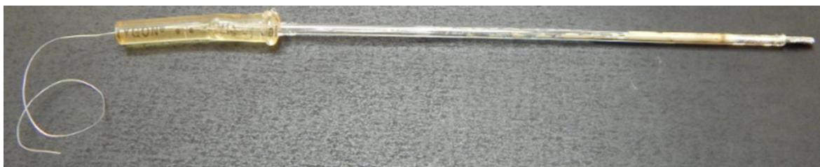
Figure 2.9. Platinum mesh based counter organic phase electrode.
