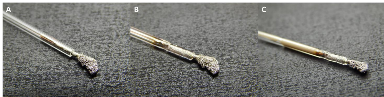
Figure 2.8. Successive steps of electrode preparation. A – Platinum mesh and wire inserted into the capillary, B – glass melted around the platinum wire and C – conductive resin placed above the wire.
