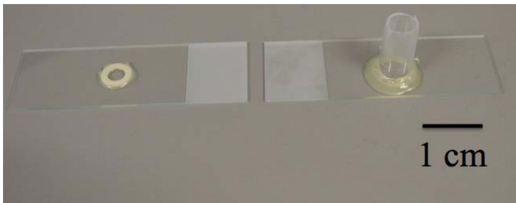
Figure 1.5 – The two typical cells used to conduct these experiments, as shown both cells are glued on a glass slide.
