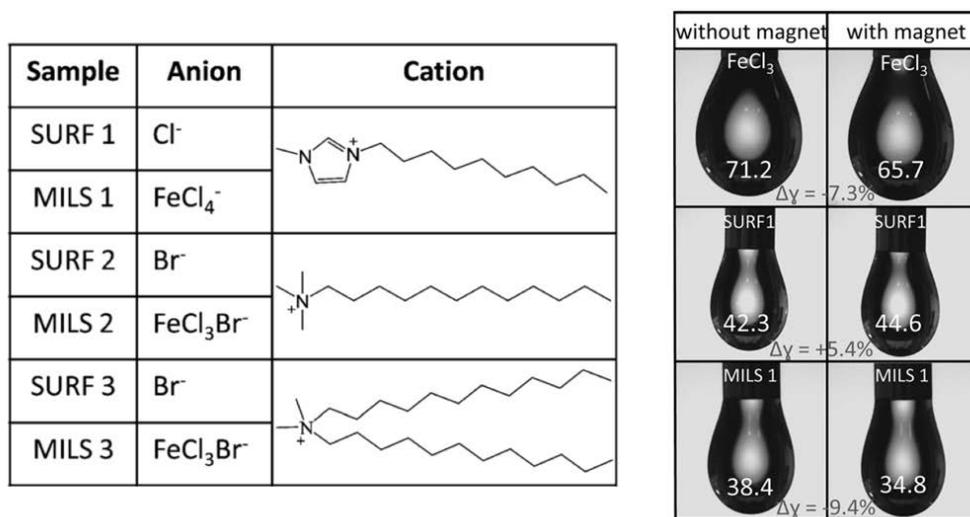
Figure. 3.1 Some example of conventional surfactants (SURF) and their magnetic surfactants (MILS) (left); Response of liquid droplets to the field from a 0.4 T NdFeB magnet. [SURF1]=20 wt%, [MILS1]=20 wt% (right)
