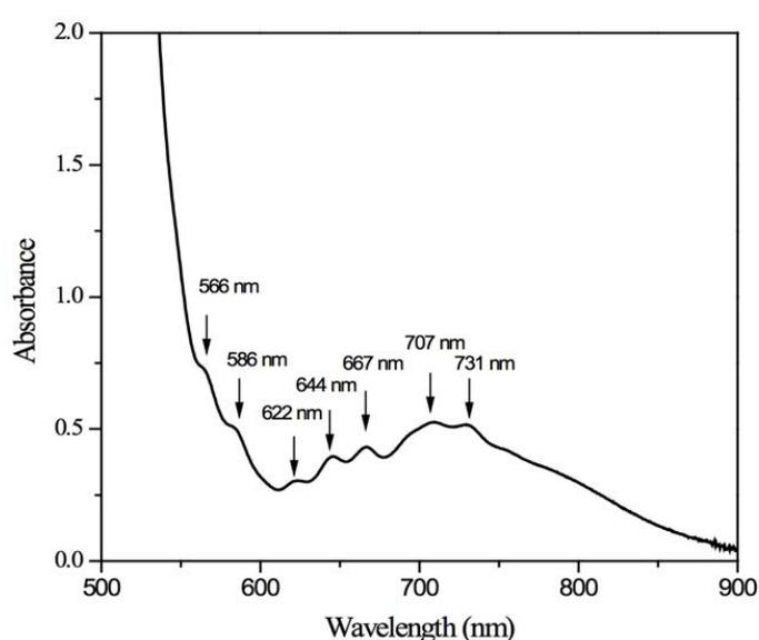
Figure 3.2.1. UV-Visible spectra of CTAF (0.1 M in acetonitrile).
