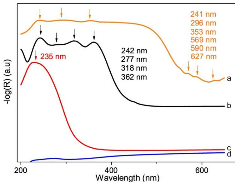
Figure 3.2.12. UV-Visible diffuse reflectance spectra of materials: (a) CTAF, (b) CTAF@SiO<sub>2</sub>(hybrid), (c)Fe@SiO<sub>2</sub>, and (d) Bare SiO<sub>2</sub>
