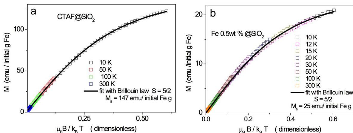
Figure 3.2.14. Magnetization of (a) the hybrid  $\text{CTAF@SiO}_2$  and (b)  $\text{Fe@SiO}_2$  samples measured at different temperatures and plotted as a function of the ratio of the magnetic field (B) to temperature (T).
