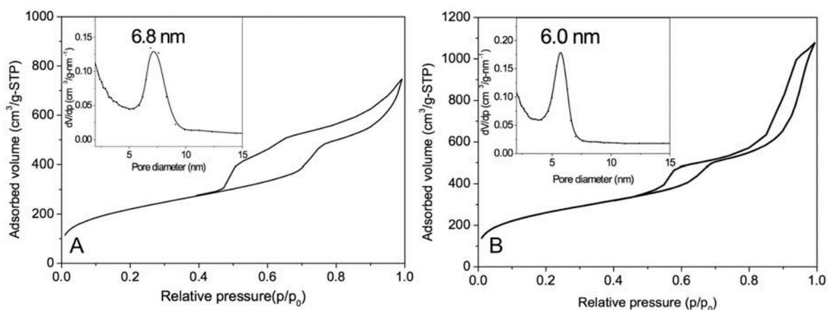
Figure 2.1.6. Nitrogen adsorption–desorption isotherm and pore size distribution (inset) of (A) CU-Mat, (B) CU-SA-Mat.
