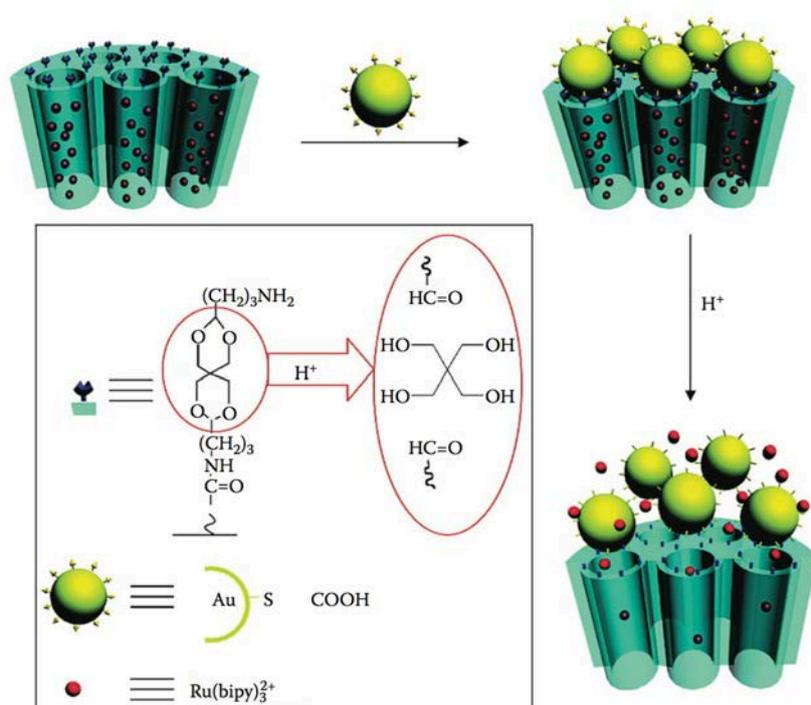
Figure 1.4. Schematic illustration of pH-responsive nanogated ensemble based on gold-capped mesoporous silica through acid-labile acetal linker.<sup>115</sup>
