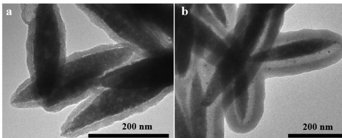
Figure 3.3.7 TEM image of Cui *et al.*'s catalyst, the yolk-shell structured Fe<sub>2</sub>O<sub>3</sub>@mesoporous SiO<sub>2</sub> composite with tuned void space size ((a) 5 nm; (b) 40 nm). Methylene blue degradation data cited in this study is the result for the material with void space of 40 nm (b).
