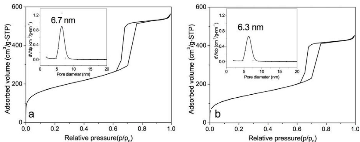
Figure 2.3.14. N<sub>2</sub> adsorption–desorption isotherms and pore size distribution (inset) of (a) SBA-15, (b) SBA-15-CU. The BET specific surface area and the mesopore volume are 638 m<sup>2</sup> g<sup>-1</sup> and 0.91 cm<sup>3</sup> g<sup>-1</sup> for (a) SBA-15, 461 m<sup>2</sup> g<sup>-1</sup> and 0.70 cm<sup>3</sup> g<sup>-1</sup> for (b) SBA-15-CU, respectively.
