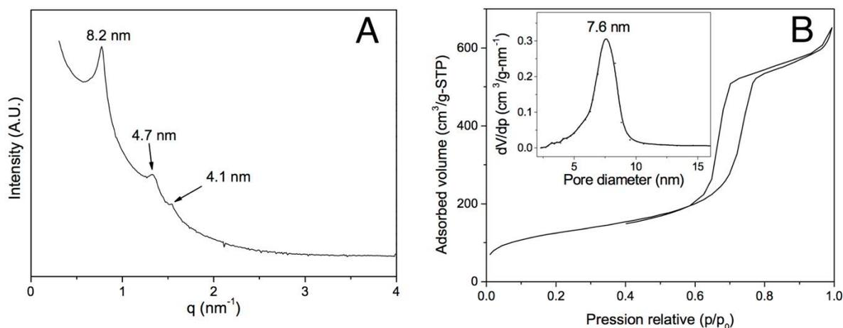
Figure 3.3.10. (A) SAXS patterns of Fe<sub>2</sub>O<sub>3</sub>@meso-macroporous silica after 5 runs; (B) N<sub>2</sub> adsorption–desorption isotherms and pore size distribution (insert) of Fe<sub>2</sub>O<sub>3</sub>@meso-macroporous silica after 5 runs.
