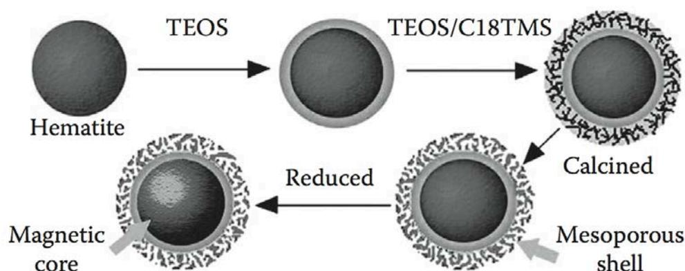
Figure 1.11. Illustration of synthesis of MFeCMS nanospheres. (C18TMS for *n*-octadecyltrimethoxysilane)<sup>142,143</sup>
