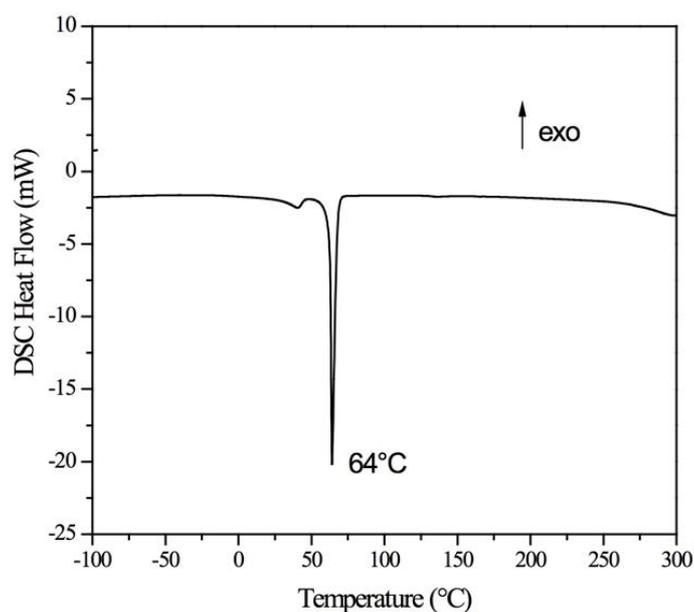
Figure 3.2.2. DSC measurement of magnetic surfactant CTAF
