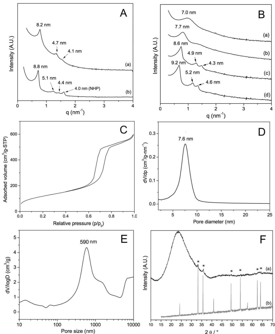
Figure 3.3.3. (A) SAXS patterns of (a) Fe<sub>2</sub>O<sub>3</sub>@meso-macroporous silica (the catalyst), (b) as-synthesized material; (B) SAXS patterns of meso-macroporous silica prepared with CTAF, (a) 3.0 wt.%, (b) 2.4 wt.%, (c) 1.2 wt.%, and (d) 0.6 wt.%; (C) N<sub>2</sub> adsorption-desorption isotherms and (D) pore size distribution of the catalyst; (E) Macropore size distribution of the catalyst; (F) (a) XRD pattern of the catalyst, (b) commercial hematite from Sigma-Aldrich.
