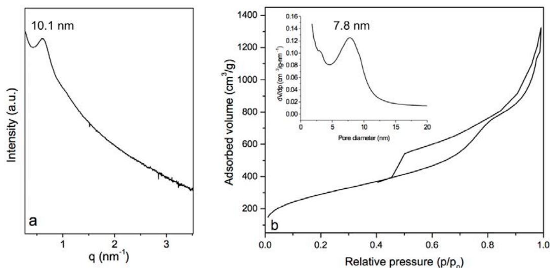
Figure 2.2.3. (a) SAXS and (b) N<sub>2</sub> adsorption-desorption isotherm with pore size distribution (inset) of hollow silica microcapsules imprinted with SLN.
