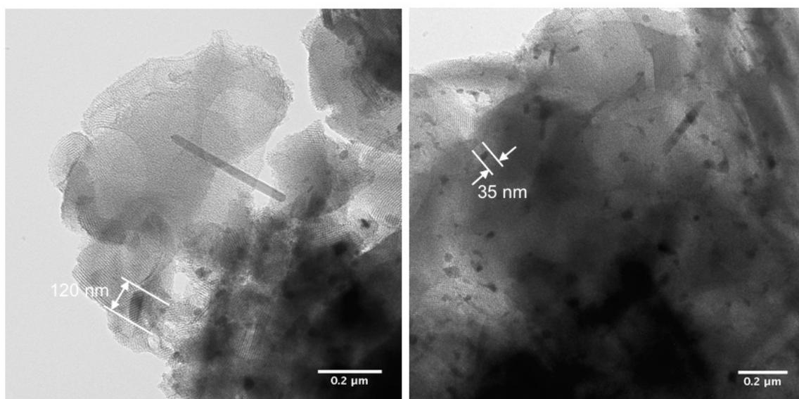
Figure 3.3.4. Two TEM images of silica material prepared using 3.0 wt.% of CTAF. It is clearly shown that the size of metallic particles (probably  $\text{Fe}_2\text{O}_3$ ) is bigger than that of the silica material prepared in the optimal condition (Figure 3.3.5A)
