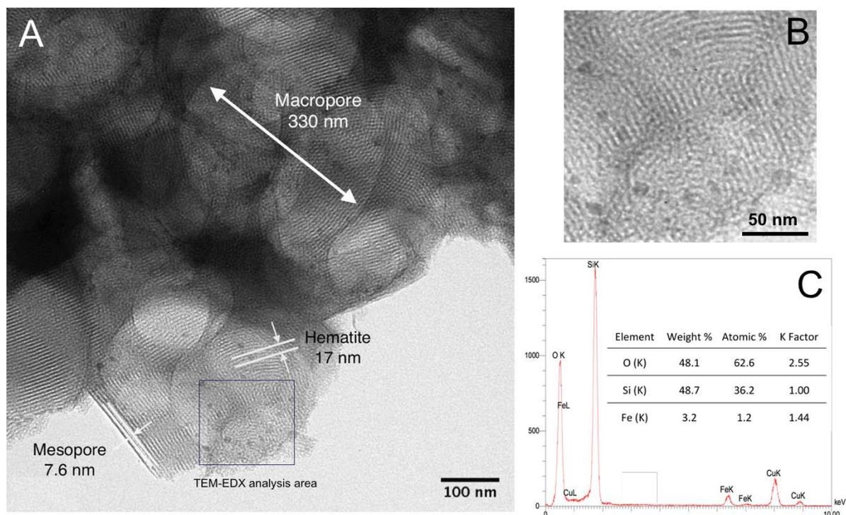
Figure 3.3.5. (A) TEM image of Fe<sub>2</sub>O<sub>3</sub>@meso-macroporous silica; (B) Zoomed image of TEM-EDX analysis area; (C) TEM-EDX analysis result.
