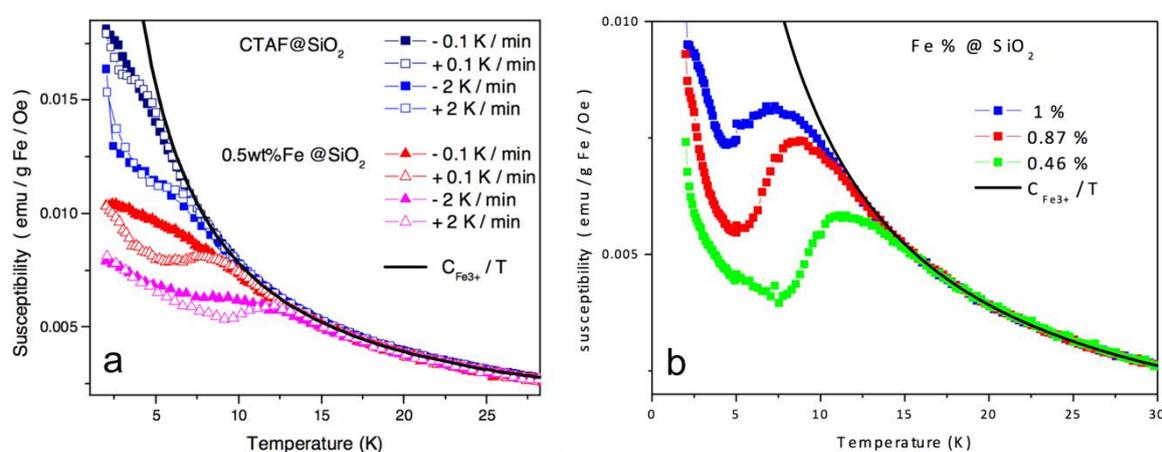
Figure 3.2.15. (a) Low temperature behaviour of  $\chi$  measured under 1T for CTAF@SiO<sub>2</sub> and 0.5 wt.% Fe@SiO<sub>2</sub>. The Curie law behaviour of  $\chi$  expected for  $S = 5/2$  Fe<sup>3+</sup> (straight line). Two rates of 0.1 and 2 K min<sup>-1</sup> with decreasing (-) or increasing (+) temperature. (b)  $\chi$  of several Fe@SiO<sub>2</sub> materials measured with increasing temperature under  $B = 1T$ .
