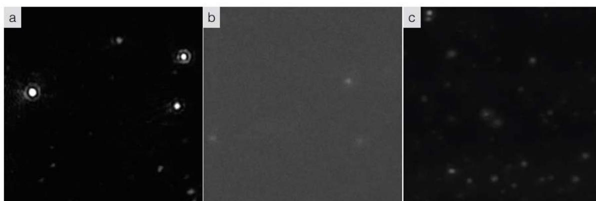
Figure 2.2.2. Captured images of Nanoparticle Tracking Analysis (NTA) for (a) CU-SLN without any filter (b) CU-SLN with fluorescence filter (c) Nile Red-SLN with fluorescence filter.
