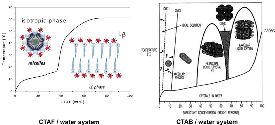
Figure 3.2.3. Concentration-temperature phase diagram of CTAF/water (left) and CTAB/water<sup>69</sup> (right) systems.
