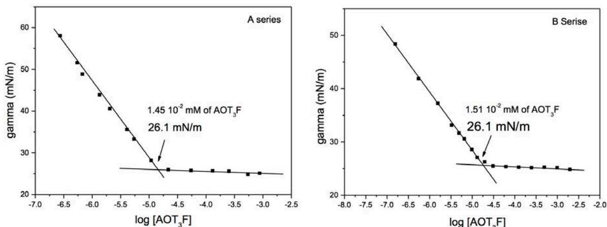
Figure 3.1.4. Critical aggregation concentration (CAC) of vesicle solutions determined using Surface tension measurements.
