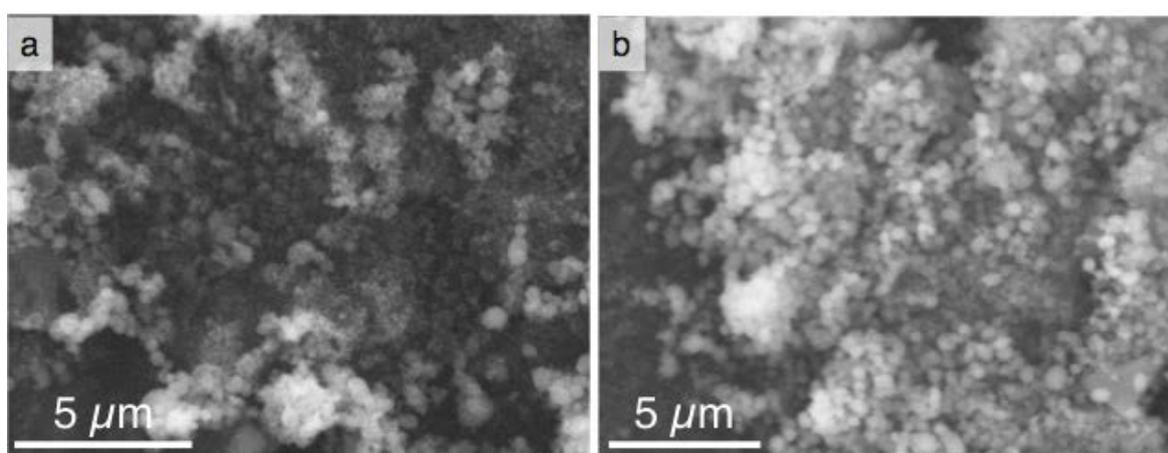
Figure 2.3.6. SEM image of (a) MCM-41, (b) MCM-41-CU-TA
