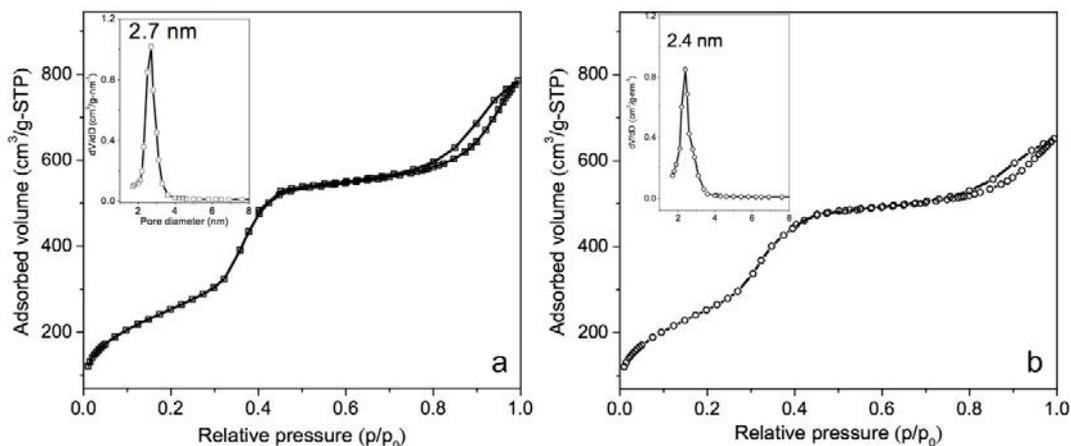
Figure 3.2.11. N<sub>2</sub> adsorption–desorption isotherm of (a) bare mesoporous silica, (b) Fe@SiO<sub>2</sub>, and their pore size distribution (inset).
