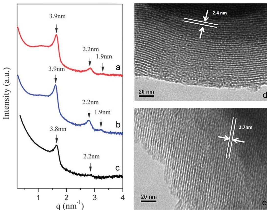
Figure 3.2.10. SAXS patterns for silica materials: (a) Fe@SiO<sub>2</sub>, (b) Bare SiO<sub>2</sub>, and (c) CTAF@SiO<sub>2</sub>; TEM micrograph of (d) Fe@SiO<sub>2</sub>, and (f) Bare SiO<sub>2</sub>.
