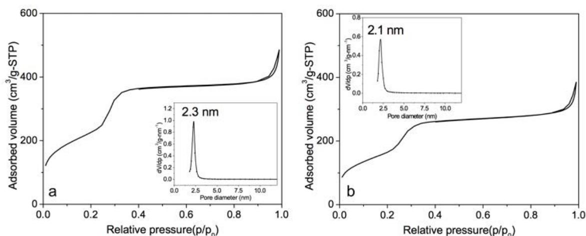
Figure 2.3.3. N<sub>2</sub> adsorption–desorption isotherms and pore size distribution (inset) of (a) MCM-41, (b) MCM-41-CU
