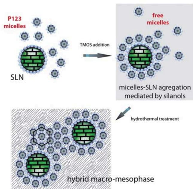
Figure 2.1.1. Proposed mechanistic scheme for the formation of macro– mesostructured silica with a hexagonal mesopore network.
