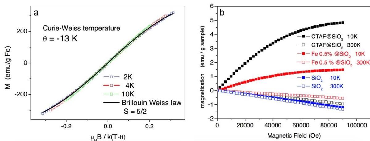
Figure 3.2.13. (a) Magnetization of magnetic surfactant, CTAF as a function of dimensions parameter  $\mu_B B / k(T-\theta)$  and its fit with the Brillouin function with  $S = 5/2$ ; (b) Magnetization of hybrid  $\text{CTAF@SiO}_2$ ,  $\text{Fe@SiO}_2$ , and bare  $\text{SiO}_2$  as a function of applied magnetic field (Oe) at 10 and 300K.
