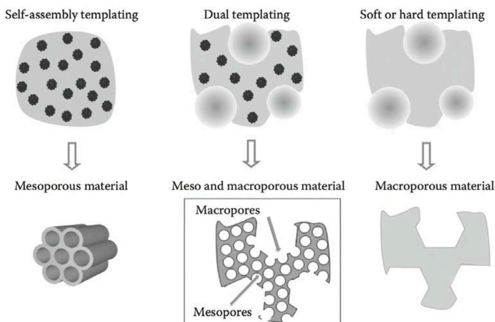
Figure 1.2. Schematic illustration of colloidal templating routes for the synthesis of porous silica materials.
