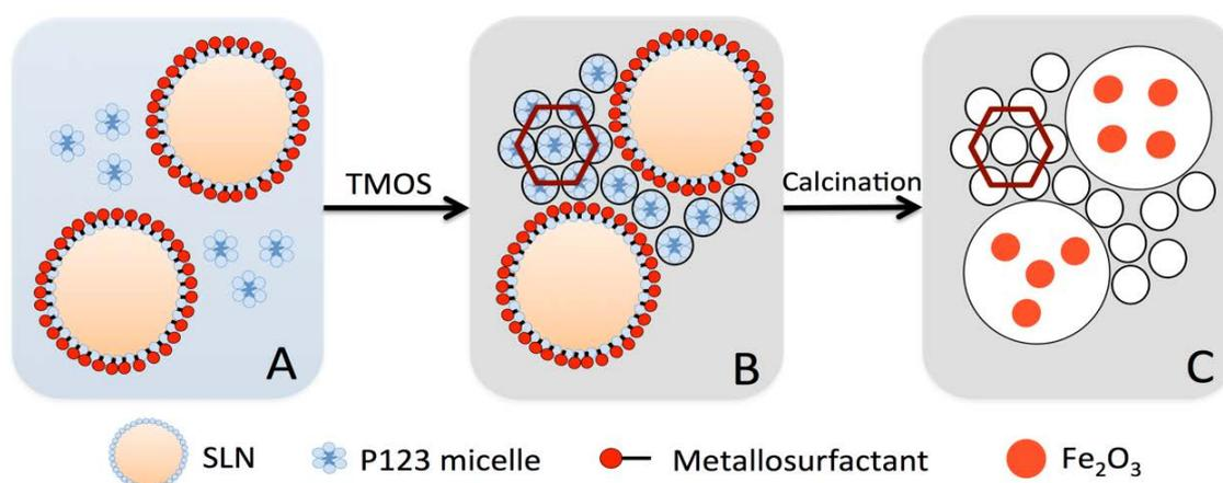
Figure 3.3.1. Synthetic strategy (not to scale): (A) CTAF-stabilized solid lipid nanoparticles (SLN) dispersed in micellar P123; (B) Silica condensation around SLN, giving hexagonally ordered mesopores; (C)  $\text{Fe}_2\text{O}_3$ @meso-macroporous silica obtained by calcination.
