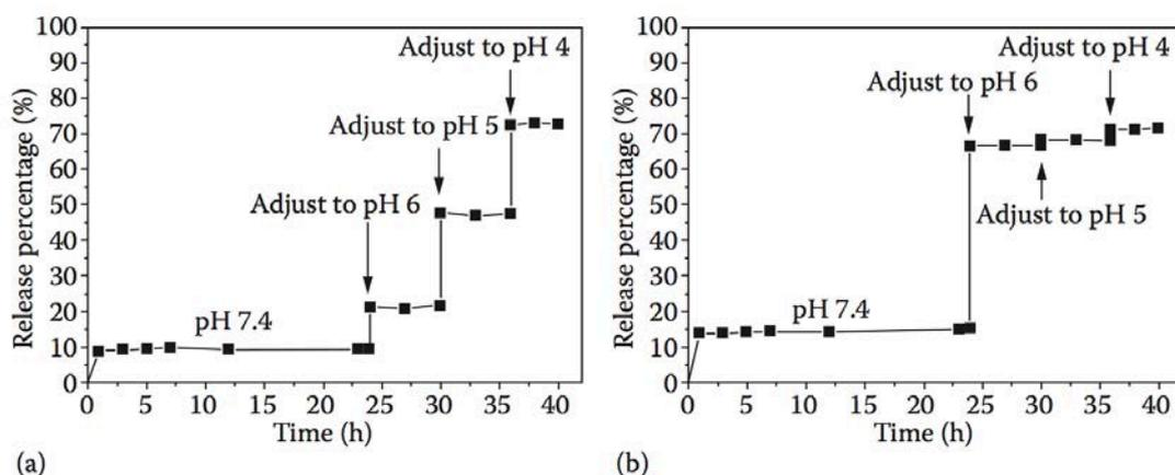
Figure 1.3. pH-responsive DOX release of  $\text{NH}_2$ -Cu-DOX (a) and  $\text{NH}_2$ -Zn-DOX (b) by acidification step by step. The AMS (Anionic surfactant templated Mesoporous Silica) nanoparticle used here was synthesized with  $\text{APS}/\text{C}_{18}\text{GluA} = 2.5$ .  $\text{Cu}(\text{CH}_3\text{COO})_2$  and  $\text{Zn}(\text{CH}_3\text{COO})_2$  have been used as metal sources.<sup>114</sup>
