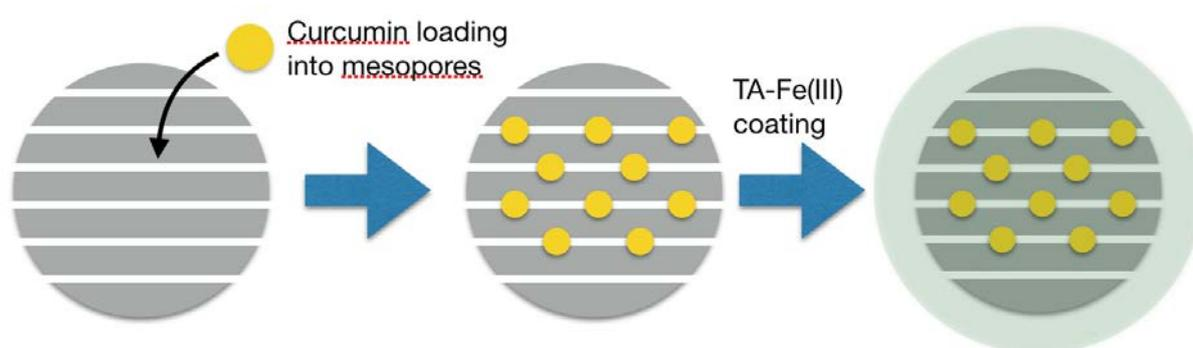
Figure 2.3.1. Synthetic pathway for curcumin loaded mesoporous silica nanoparticles (MSN) using tannic acid-Fe(III) complex.
