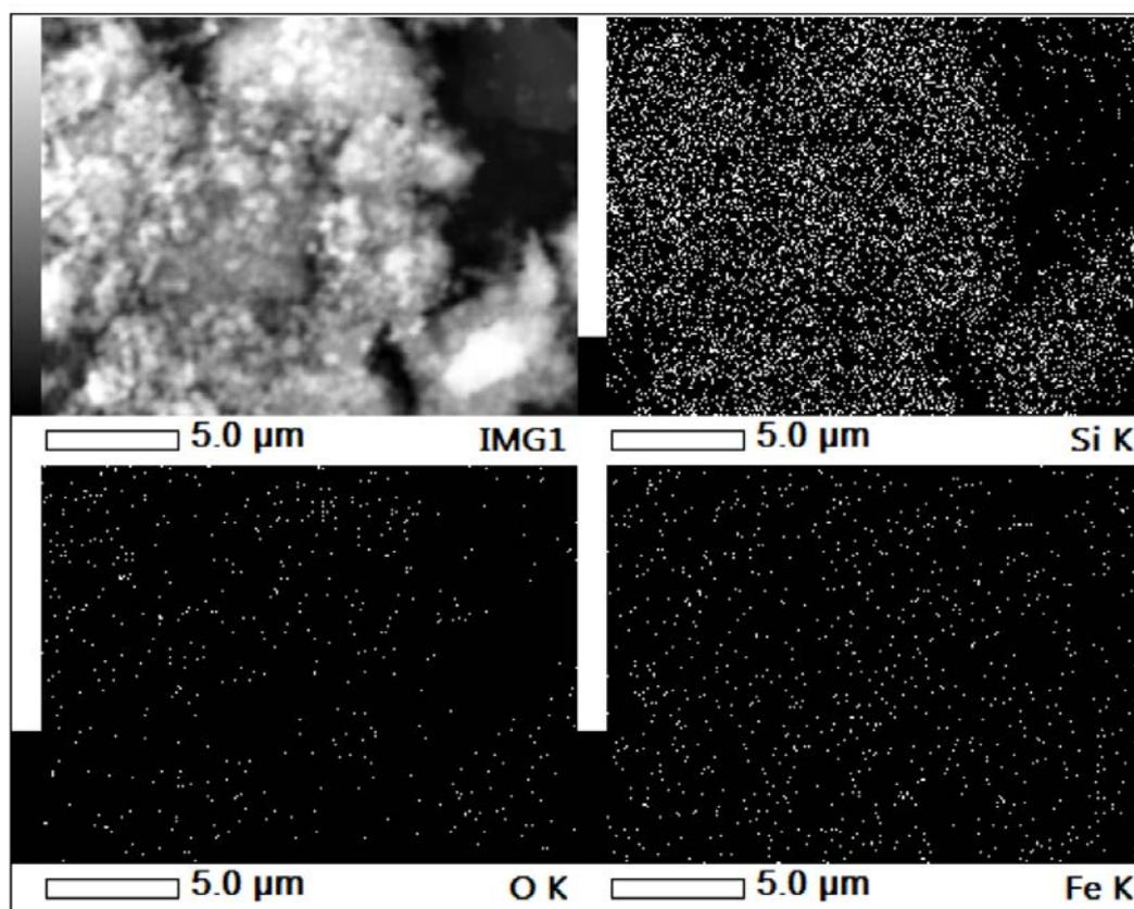
Figure 2.3.7. SEM-EDS mapping image of MCM-41-CU-TA
