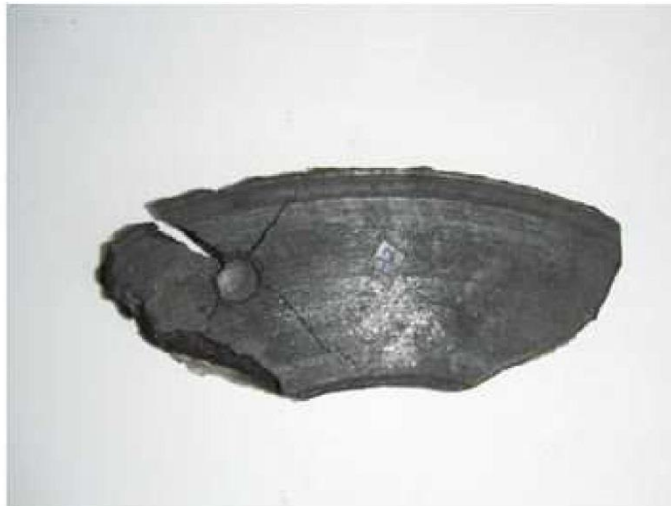
Figure 8: Formulation 13 after Brinell hardness test
