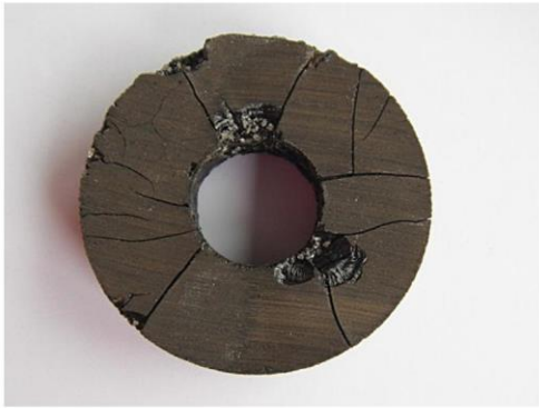
Fig. 1. 150% Alu 24, quebracho resin (Sample 9).
