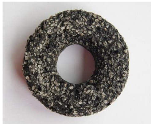
Fig. 3. 150% Alu 16, quebracho resin without water addition, with tung oil and glyoxal and with pTSA (Sample 15).
