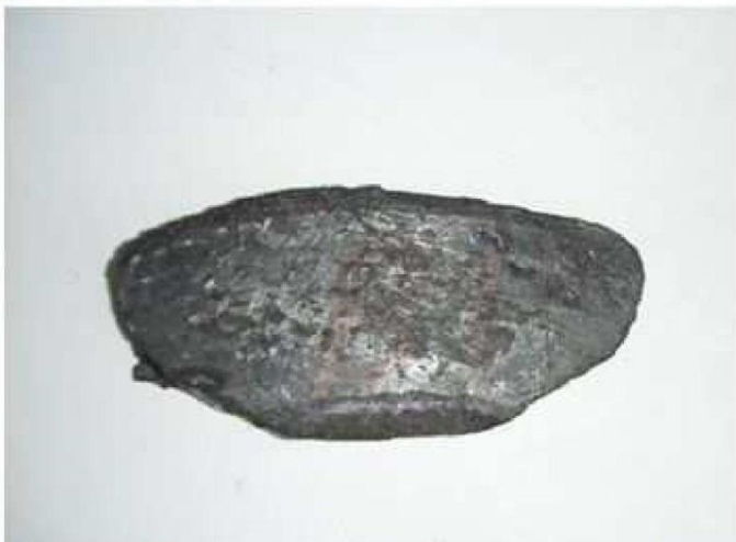
Figure 2: Formulation 3 after braking test
