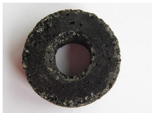
Fig. 4. 200% Alu 16, quebracho resin without water addition, with linseed oil and with pTSA (Sample 17).
