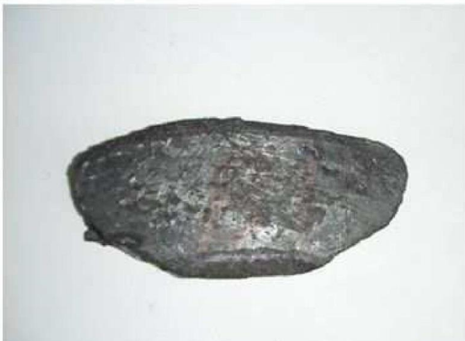
Figure 2: Formulation 3 after braking test
