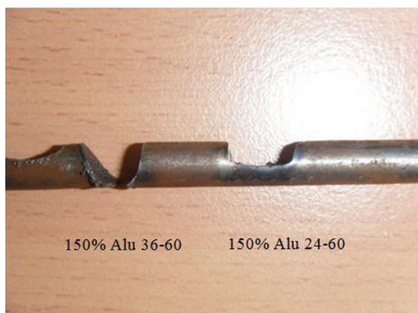
Fig. 6. Results of the tests of the tannins resin bonded grinding discs: 150% of mix of Alu 24, 36 and 60.
