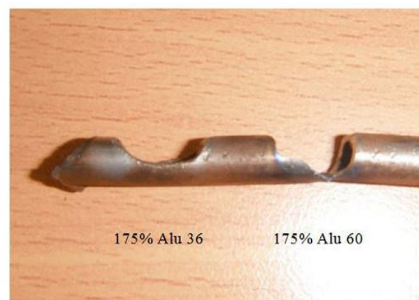
Fig. 5. Results of the tests of the tannins resin bonded grinding discs: 175% of Alu 36 and 60.
