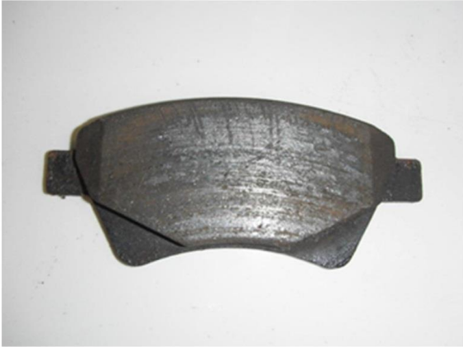
Figure 1: Commercial brake pad after braking test
