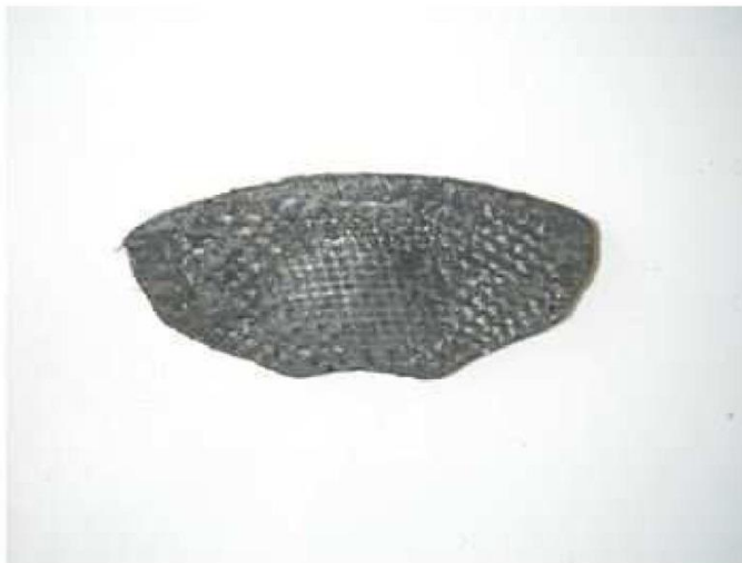
Figure 4: Formulation 7 after braking test
