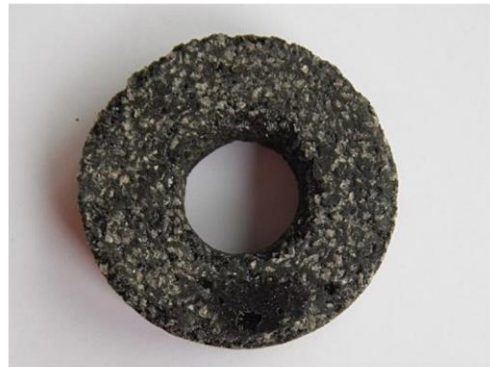
Fig. 2. 150% Alu 16, quebracho resin without water addition and with pTSA (Sample 13).
