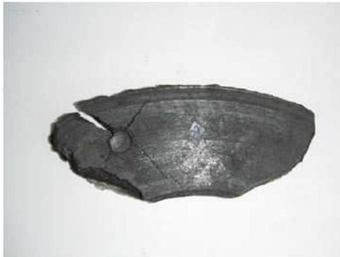
Figure 8: Formulation 13 after Brinell hardness test
