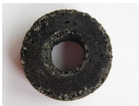
Fig. 4. 200% Alu 16, quebracho resin without water addition, with linseed oil and with pTSA (Sample 17).
