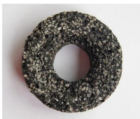
Fig. 3. 150% Alu 16, quebracho resin without water addition, with tung oil and glyoxal and with pTSA (Sample 15).
