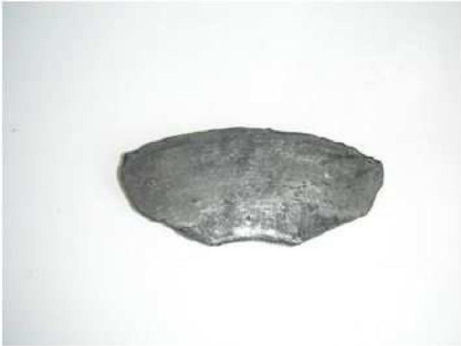
Figure 6: Formulation 12 after braking test
