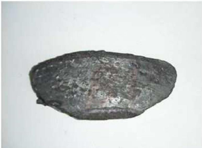
Figure 2: Formulation 3 after braking test
