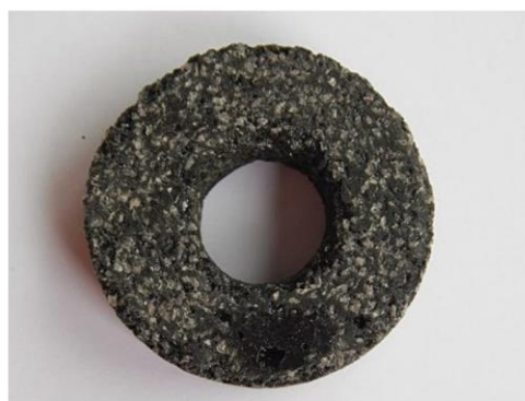
Fig. 2. 150% Alu 16, quebracho resin without water addition and with pTSA (Sample 13).
