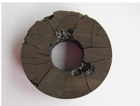
Fig. 1. 150% Alu 24, quebracho resin (Sample 9).
