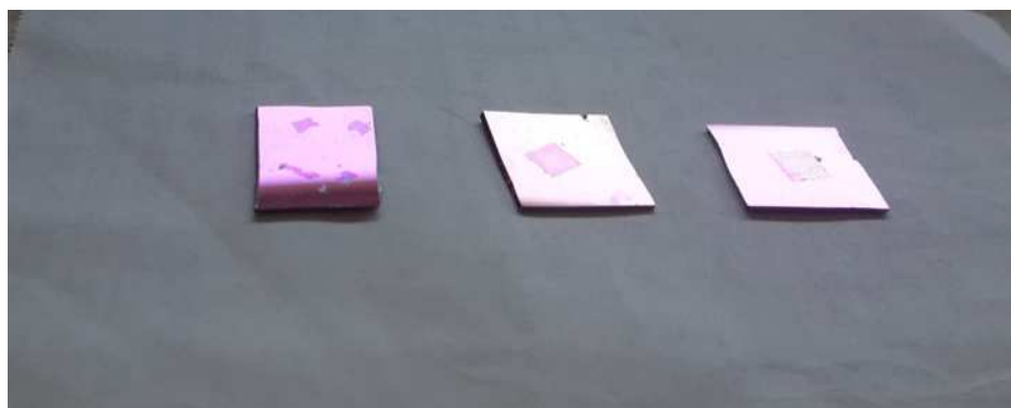
Figure 4.21 Photograph of graphene sheets separated and deposited onto a silicon wafer. Growth conditions: 850 °C for 5 min with various methane partial pressure of (left) 0.1 atm, (center) 0.2 atm and (right) 0.3 atm.
