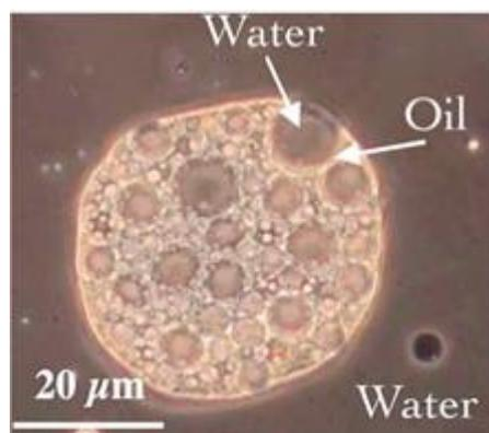
Figure 1-7: Micrographs of droplets of multiple emulsions.<sup>29</sup>
