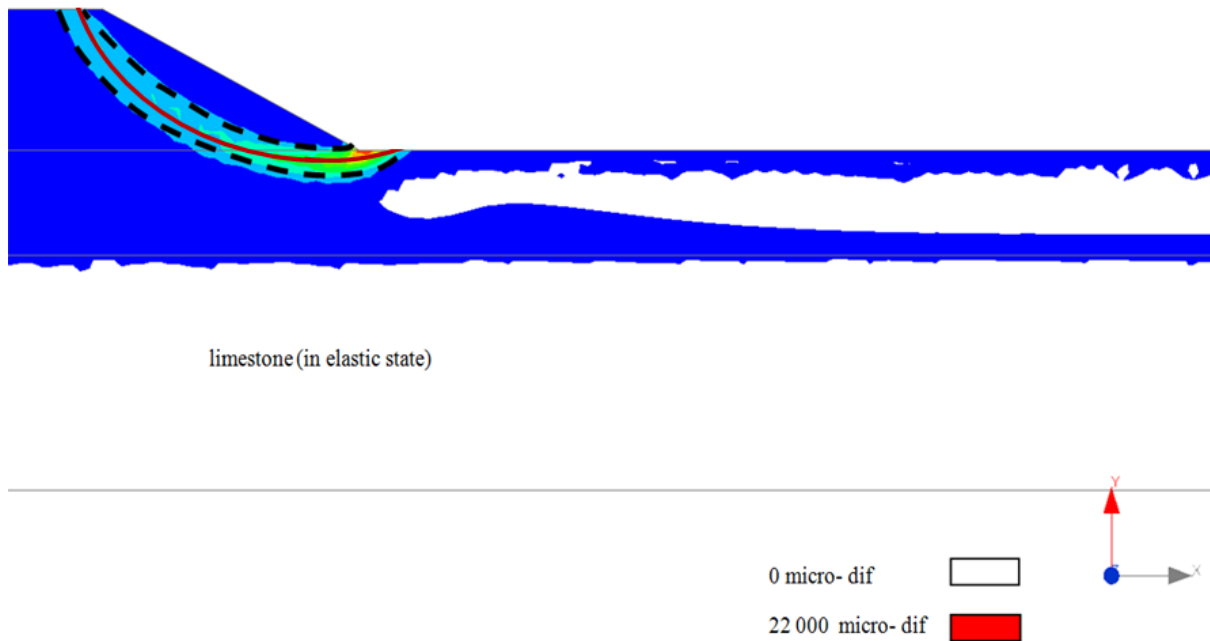
Figure 73 Isovalues of the plastic strain norm for the dike of Val d'Orléans by using the c-phi reduction method in CESAR with finite element dimensions equal to 0.5 m. The dotted lines refer to the range of potential failure surface, while the red line refers to the failure surface got from the ordinary method (TALREN software).
