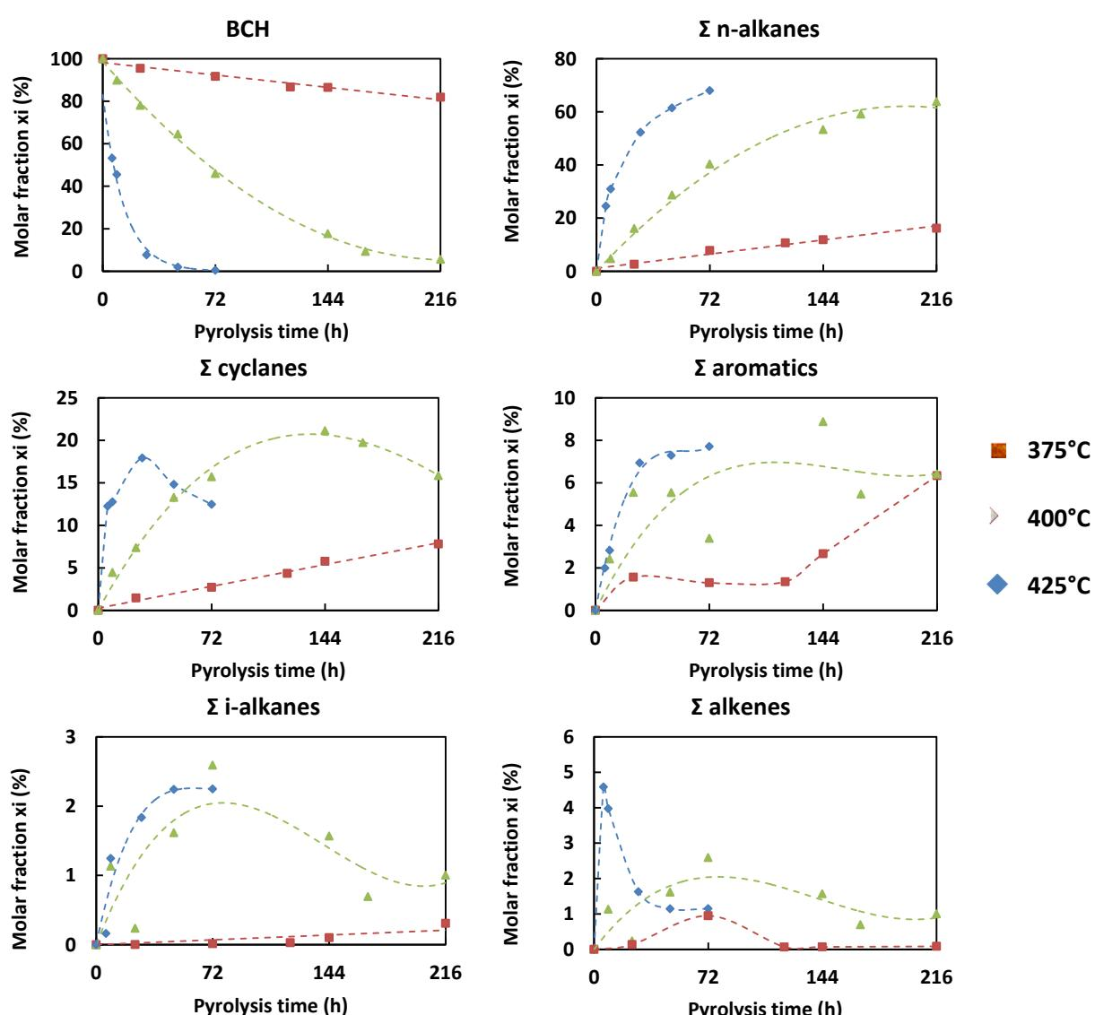
Figure 2.5 Evolution of chemical families vs temperature at 100 bar (dotted lines suggest trends)
