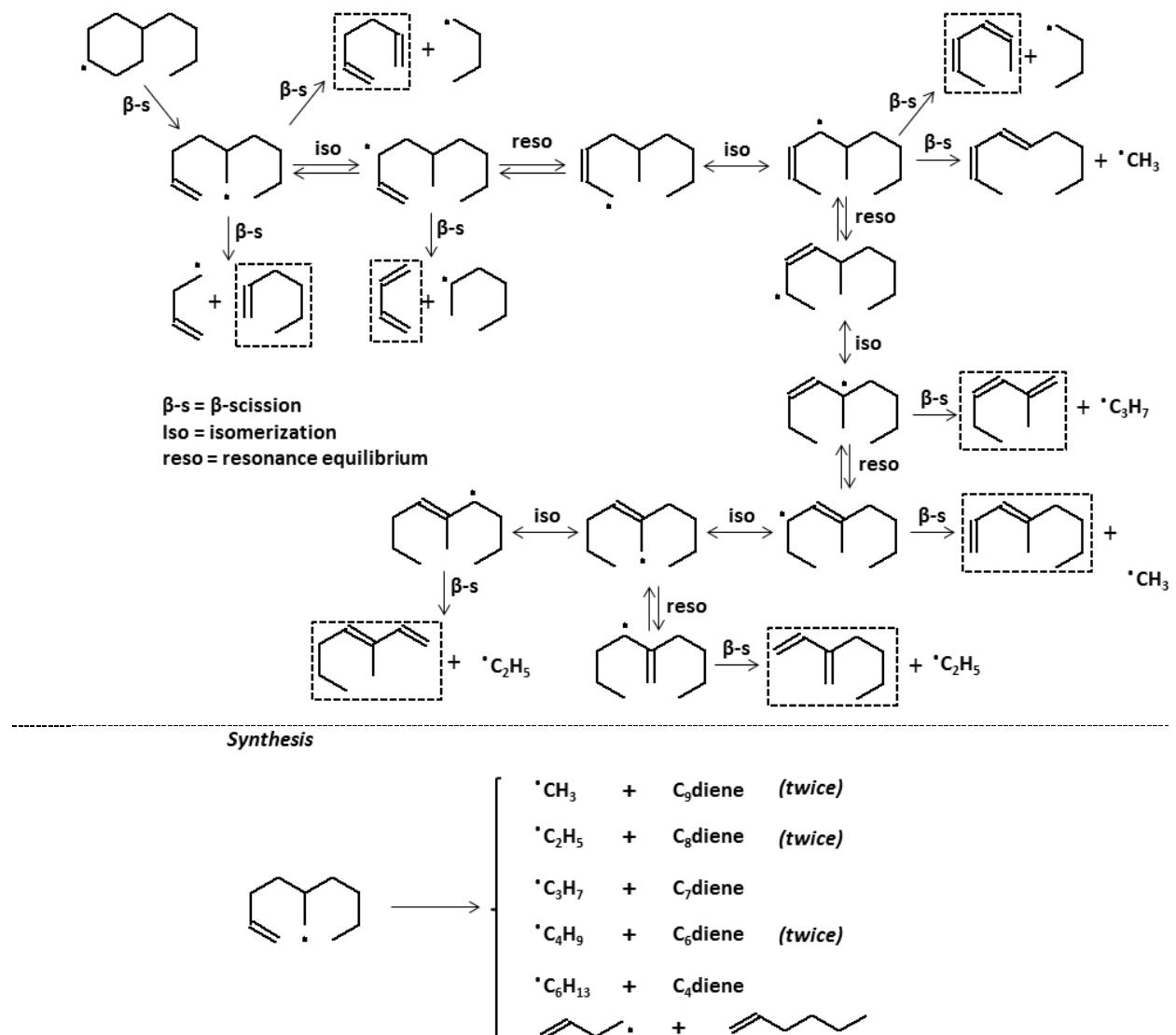
Figure 3.3 Decomposition pathways of an alkenyl radical
