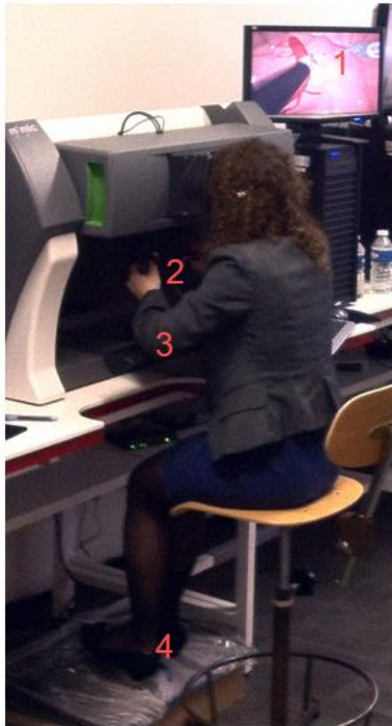
Figure 3-1 : Trainer's check points on the trainee: 1. operation procedure on the monitor ; 2. the position of joysticks ; 3. the position of forearms ; 4. the pedal using .
