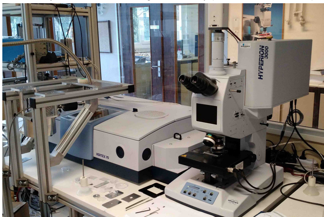
Figure 3-7: A photo of the Bruker Vertex 70 spectrometer coupled with a Bruker Hyperion 3000 FTIR-microscope.
