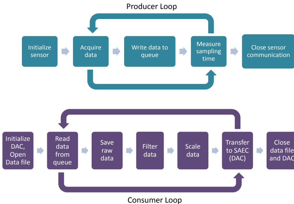
Figure 3.7 – Schematic of LabView data acquisition application
