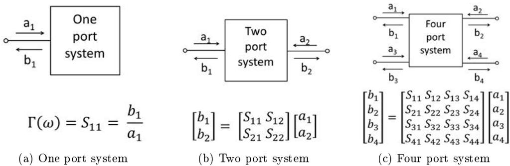
Figure 2.6 – S-parameters of one-, two- and four-port systems
