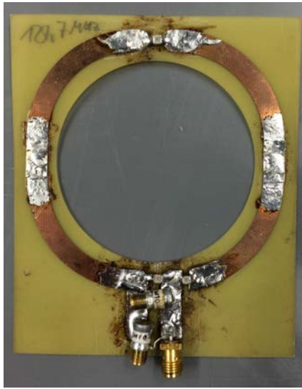
(a) 127.7 MHz single loop coil with 75 mm diameter and 8 mm conductor width
