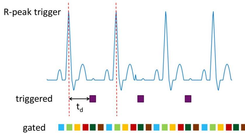
Figure 1.12 – Triggering and gating in cardiac imaging: The trigger point is defined by the R-peak of the ECG. After a defined trigger delay time  $t_d$  the image is acquired. In cardiac gating the image acquisition is performed continuously and reordered retrospectively (various cardiac phases are illustrated in different colors)
