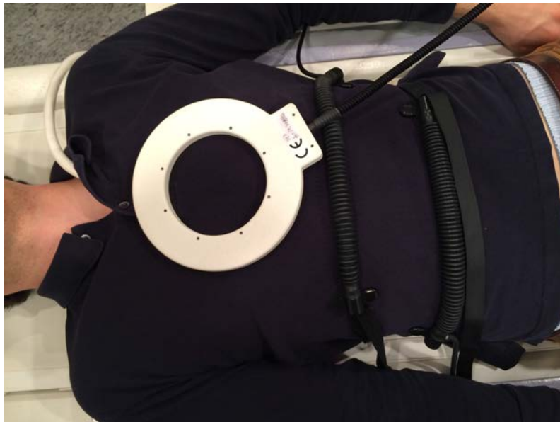
Figure 6.8 – Setup of loop coil measurement. Coil fixation is removed for visualization. ECG, respiratory belts at the chest and at the abdomen are used for this measurement
