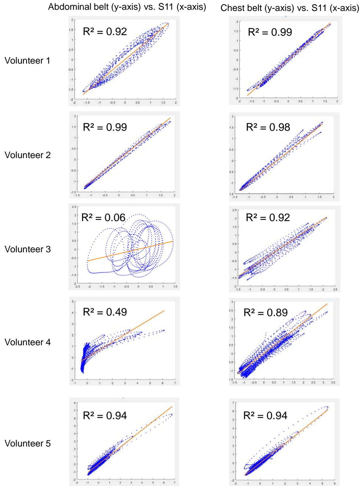
Figure 6.9 – Correlation between the coil S11 data and the abdominal belt signal (left), and between the coil S11 data and the chest belt signal (right), for each volunteer
