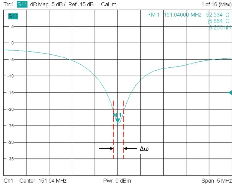
Figure 2.7 – Magnitude of  $S_{11}$  coefficient of a coil measured with a VNA; Marker M1 indicates the resonant frequency  $\omega_0$  and  $\Delta\omega$  the 3 dB bandwidth. The ratio of both values is the quality factor  $Q$  (Eq. 2.24)
