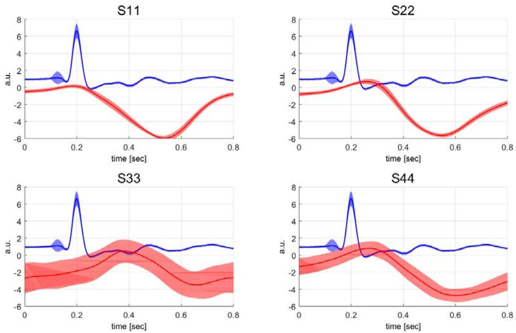
Figure 6.20 – Cardiophysiologic signal of reflection coefficients of 4-ch coil during free-breathing. A higher standard deviation is observed in  $S_{33}$  and  $S_{44}$  signal, mainly due to the larger distance to the heart
