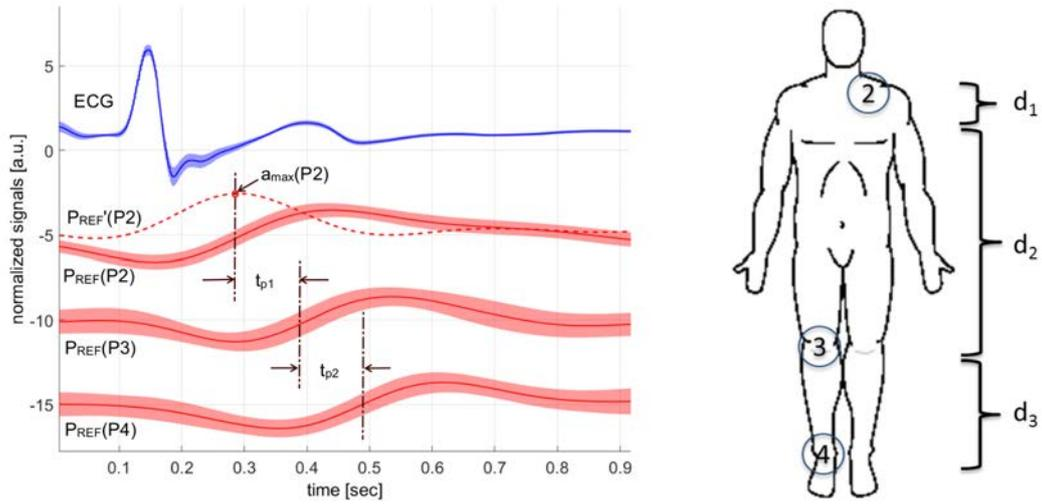
Figure 6.4 – Time points and distances for PWV calculations. left: time points definitions is performed by evaluating the maximum of the first derivative  $a_{max}$ , shown here for the curve on position 2 ( $P_{REF}(P2)$ ); right: distances between measurement positions, see text for detailed explanation
