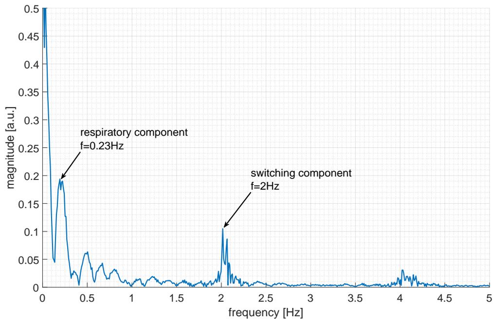
Figure 5.10 – FFT of power signal of mode frequency;  $f=0.23\text{Hz}$  corresponds to respiration frequency of 14cycles/minute;  $f=2\text{Hz}$  reflects switching frequency
