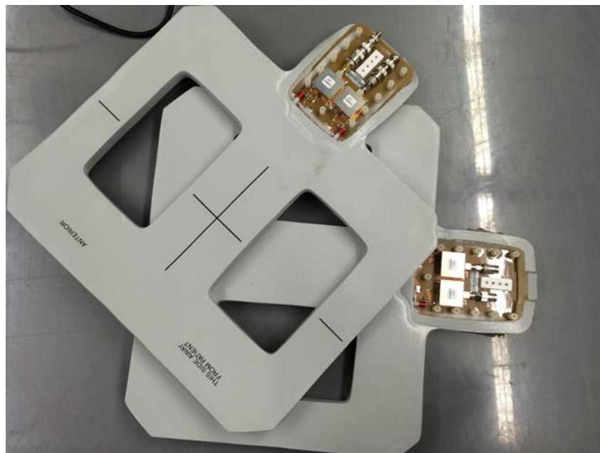
Figure 6.16 – 1.5T four channel cardiac coil; Coil cover is removed and direct connections to the coil are visible
