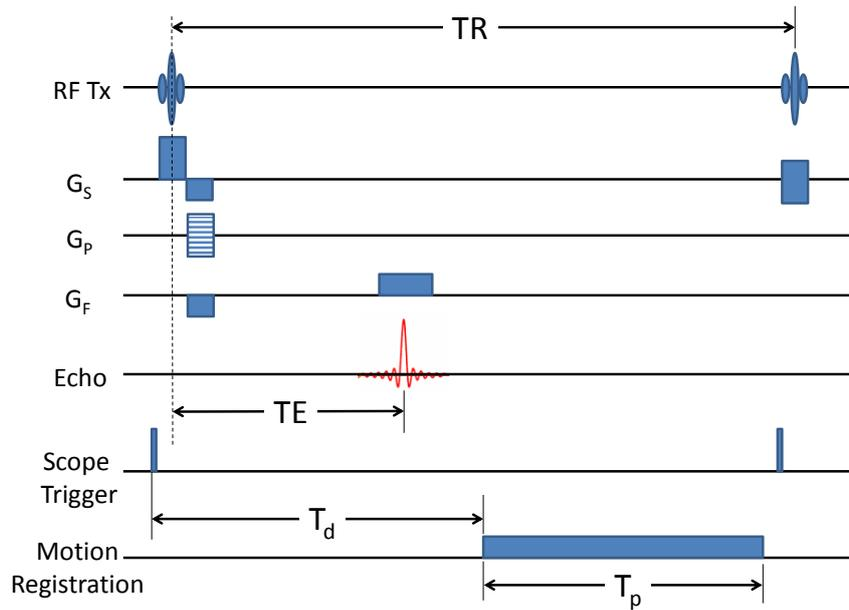
Figure 5.9 – Gradient echo sequence timing with switch activation; RF = RF excitation, G<sub>S</sub> = slice selective gradient, G<sub>P</sub> = phase encoding gradient, G<sub>F</sub> = frequency encoding gradient, Echo = receive signal, TE = Echo time, Scope trigger = trigger pulse of MR system, T<sub>d</sub> = trigger delay time, T<sub>p</sub> = switch activation time
