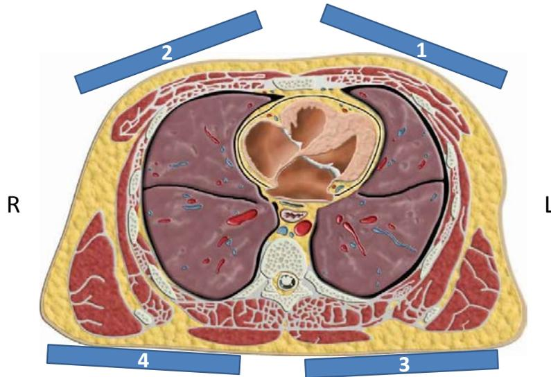
Figure 6.17 – Schematic of the coil element positions on the volunteer
