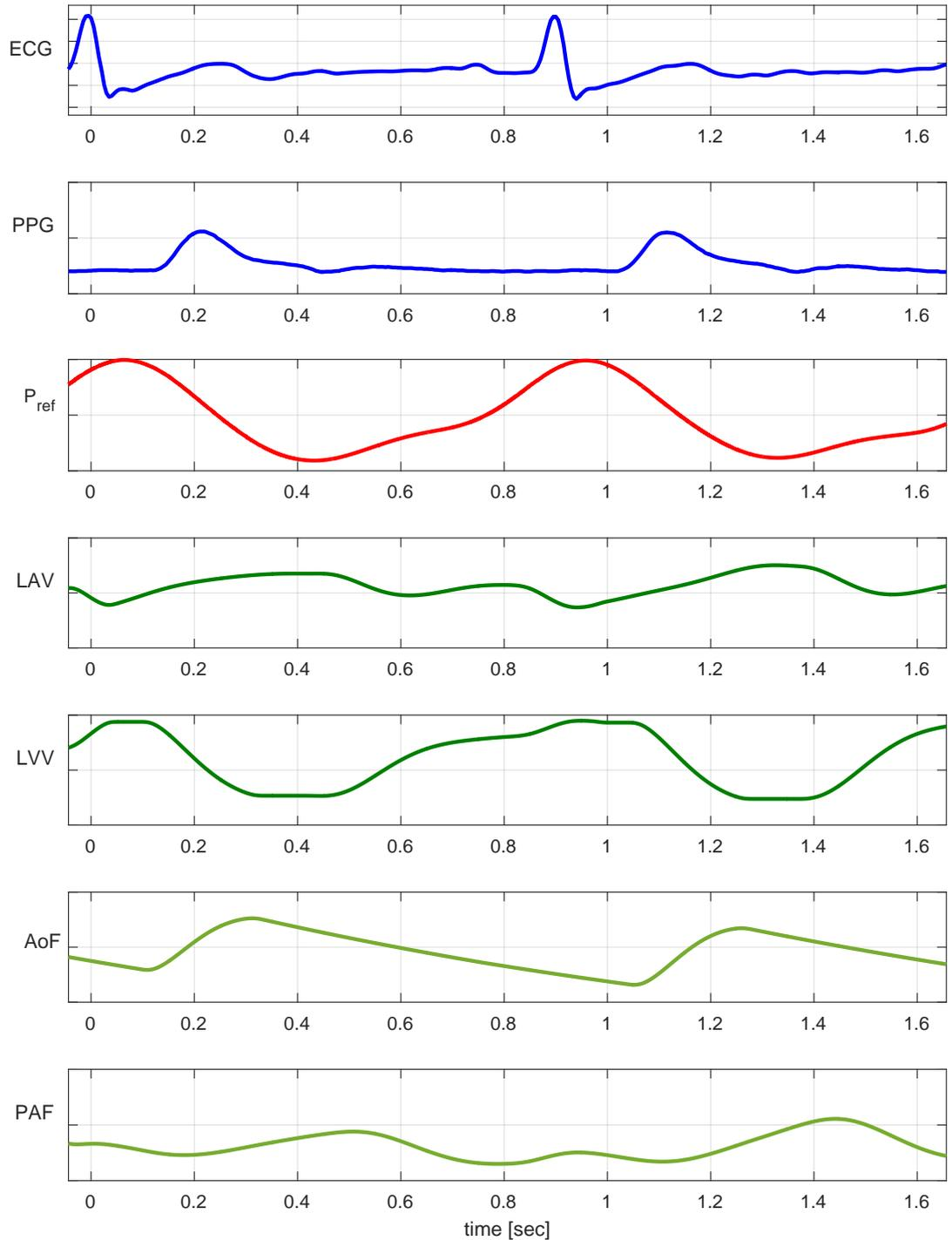
Figure 6.6 – Comparison of experimental results with simulated data of CircAdapt. ECG = electrocardiogram of MRI system, PPG = pulseplethysmograph of MRI system,  $P_{ref}$  = measured reflected power of coil, LVV = left ventricular volume, LAV = left atrial volume, AoF = aortic flow, PAF = pulmonary artery flow. y-axis values normalized in arbitrary units
