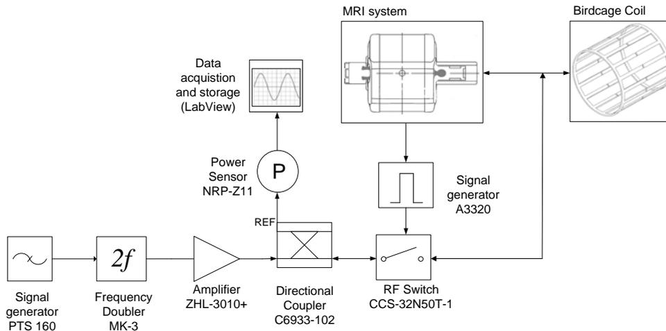
Figure 3.4 – Schematic of switch setup for motion acquisition on birdcage coil modes. The switch is controlled by an delayed trigger pulse of a pulse generator and disconnects the measurement system during excitation and image acquisition
