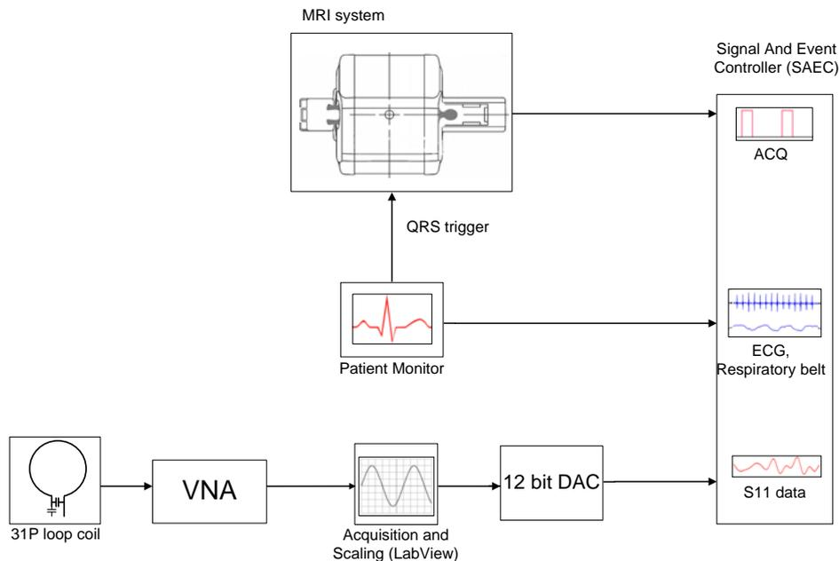
Figure 3.5 – Schematic of motion acquisition setup with VNA
