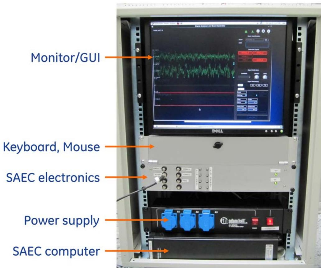
Figure 3.2 – Mobile SAEC at GRC Munich: All components are mounted in a 19 inch rack. Data transfer is available through USB and TCP/IP (for saved data only)
