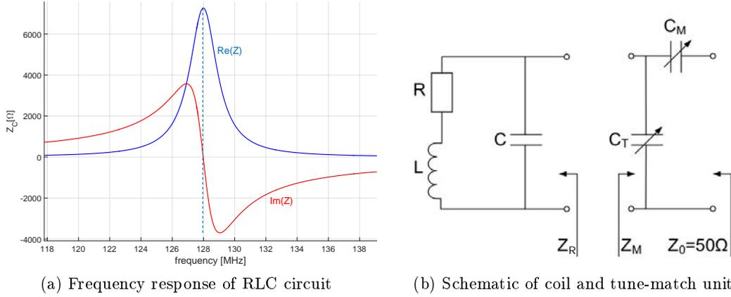
Figure 2.1 – a) Real (blue) and imaginary (red) part of frequency dependent impedance of coil circuit. Resonance frequency is at 128MHz (dashed line) with  $R=2\Omega$ ,  $L=150\text{nH}$ ,  $C=10\text{pF}$ . b) Schematic of coil circuit (left) and tuning and matching network (right). The aim of this network is to adjust the impedance of the coil to the system impedance of  $Z_0 = 50\Omega$
