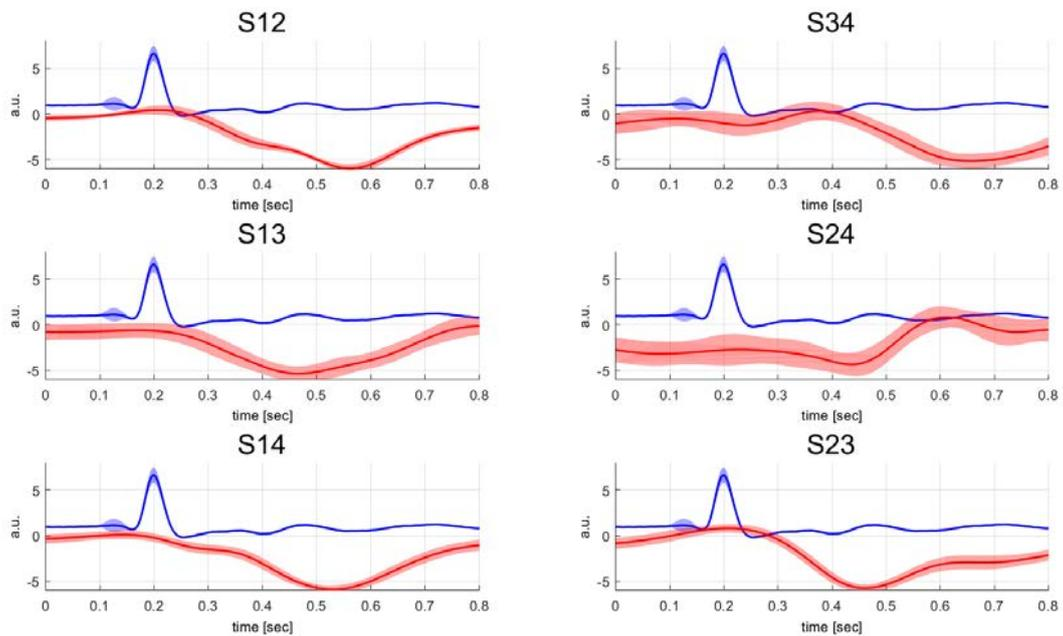
Figure 6.21 – Cardiophysiologic signal of transmission coefficients of 4-ch coil during free-breathing; Signal along the heart axis ( $S_{14}$  and  $S_{23}$ ) are more accurate and show lower standard deviation
