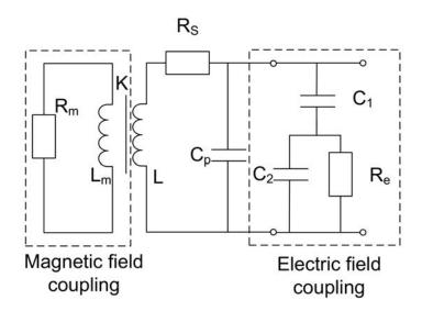
Figure 2.2 – Equivalent circuit for sample losses [104]; Magnetic field effects are represented by  $R_m$ ,  $L_m$  and K, losses caused by electric field interactions are represented by  $R_e$ ,  $C_1$  and  $C_2$
