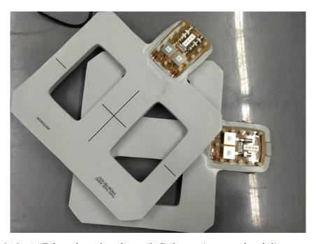
Figure 6.16 - 1.5T four channel cardiac coil; Coil cover is removed and direct connections to the coil are visible
