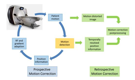
Figure 1.11 – Schematic of prospective and retrospective motion correction. Both methods are independent motion correction solutions, however they can be combined for enhanced image correction. Position information gathering by motion detection techniques is relevant for both methods
