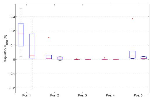
Figure 6.2 – Q-ratios for respiratory filtered signal on six volunteers at different positions; left bar: results of 64 MHz coil, right bar: results of 128 MHz coil
