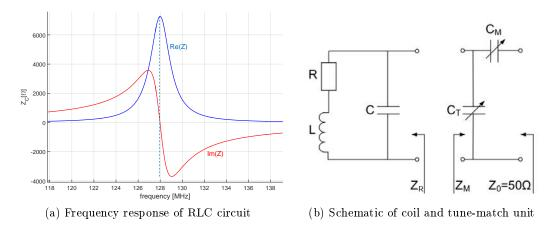
Figure 2.1 – a) Real (blue) and imaginary (red) part of frequency dependent impedance of coil circuit. Resonance frequency is at 128MHz (dashed line) with R=2 $\Omega$ , L=150nH, C=10pF. b) Schematic of coil circuit (left) and tuning and matching network (right). The aim of this network is to adjust the impedance of the coil to the system impedance of  $Z_0 = 50\Omega$
