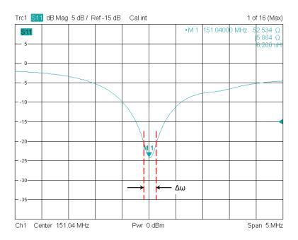
Figure 2.7 – Magnitude of S11 coefficient of a coil measured with a VNA; Marker M1 indicates the resonant frequency  $\omega_0$  and  $\Delta\omega$  the 3 dB bandwidth. The ratio of both values is the quality factor Q (Eq. 2.24)
