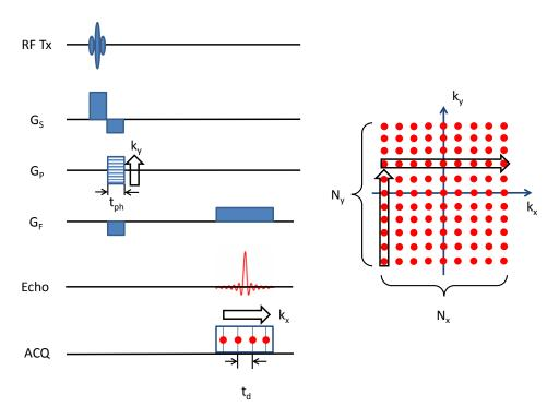
Figure 1.3 – Schematic of a MRI pulse sequence with k-space sampling; RF Tx = RF excitation,  $G_S$  = slice selective gradient,  $G_P$  = phase encoding gradient,  $G_F$  = frequency encoding gradient, Echo = receive signal, ACQ = acquisition window,  $N_x$ ,  $N_y$  = k-space matrix size,  $t_{ph}$  = phase encoding duration,  $t_d$  = dwell or sampling time
