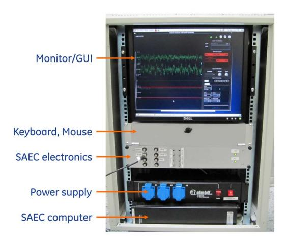
$\begin{tabular}{ll} Figure~3.2-Mobile~SAEC~at~GRC~Munich:~All~components~are~mounted~in~a~19~inch~rack.\\ Data~transfer~is~available~through~USB~and~TCP/IP~(for~saved~data~only) \end{tabular}$
