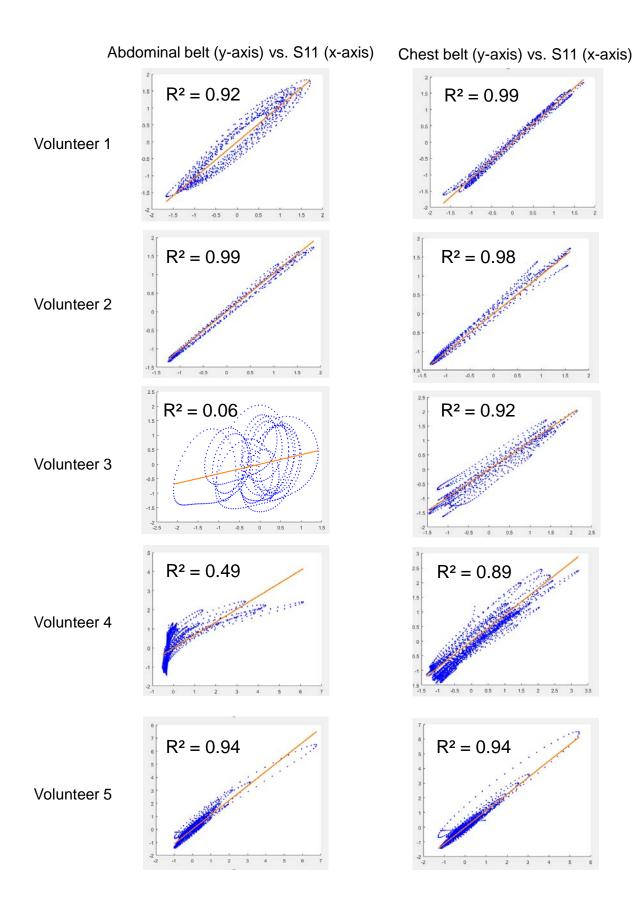
Figure 6.9 – Correlation between the coil S11 data and the abdominal belt signal (left), and between the coil S11 data and the chest belt signal (right), for each volunteer
