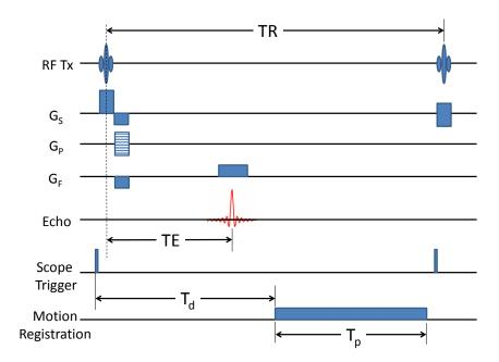
Figure 5.9 – Gradient echo sequence timing with switch activation; RF = RF excitation,  $G_S$  = slice selective gradient,  $G_P$  = phase encoding gradient,  $G_F$  = frequency encoding gradient, Echo = receive signal, TE = Echo time, Scope trigger = trigger pulse of MR system,  $T_d$  = trigger delay time,  $T_p$  = switch activation time
