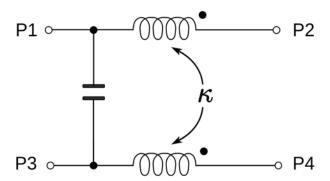
Figure 2.8 – Schematic of a directional coupler: The power of the main line between P1 and P2 is coupled according to the coupling factor  $\kappa$  to a secondary line providing a attenuated forward (P3) and reflected (P4) power levels
