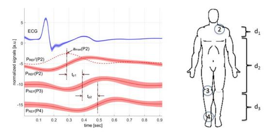
Figure 6.4 – Time points and distances for PWV calculations. left: time points definitions is performed by evaluating the maximum of the first derivative  $a_{max}$ , shown here for the curve on position 2 ( $P_{REF}(P2)$ ; right: distances between measurement positions, see text for detailed explanation
