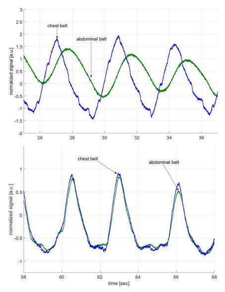
Figure 1.7 – Belt signal of two different breathing pattern; top: chest focused breathing with a phase shift in the abdominal belt; bottom: abdomen focused breathing with both belts in phase
