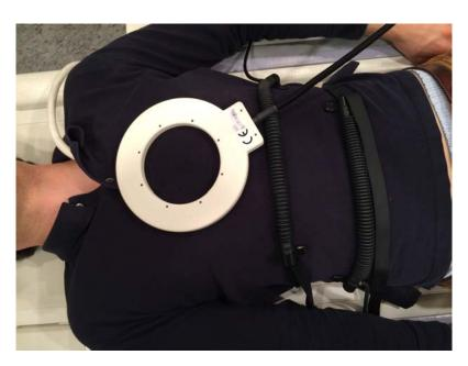
Figure 6.8 – Setup of loop coil measurement. Coil fixation is removed for visualization. ECG, respiratory belts at the chest and at the abdomen are used for this measurement
