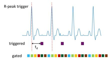
Figure 1.12 – Triggering and gating in cardiac imaging: The trigger point is defined by the R-peak of the ECG. After a defined trigger delay time  $t_{\rm d}$  the image is acquired. In cardiac gating the image acquisition is performed continuously and reordered retrospectively (various cardiac phases are illustrated in different colors)
