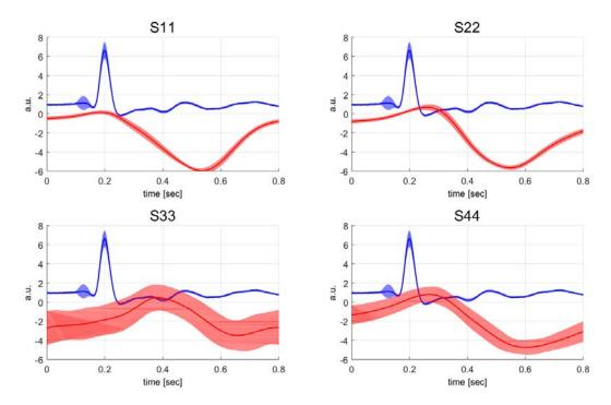
$\begin{array}{c} {\rm Figure~6.20-Cardiophysiologic~signal~of~reflection~coefficients~of~4-ch~coil~during~free-}\\ {\rm breathing.~A~higher~standard~deviation~is~observed~in~S_{33}~and~S_{44}~signal,}\\ {\rm mainly~due~to~the~larger~distance~to~the~heart} \end{array}$
