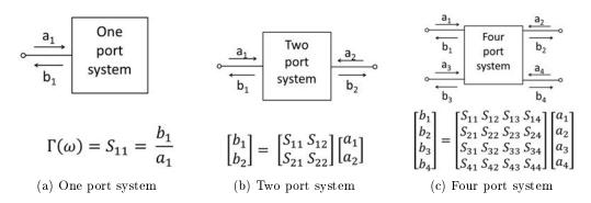
Figure 2.6 – S-parameters of one-, two- and four-port systems
