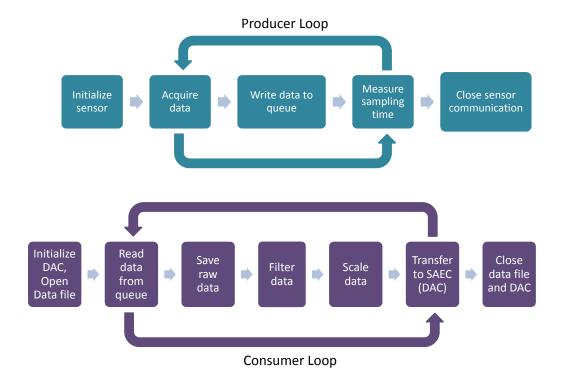
Figure 3.7 – Schematic of LabView data acquistion application
