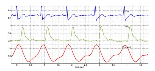
Figure 6.5 – Bandpass-filtered signal on position 1 in comparison with ECG and PPG
