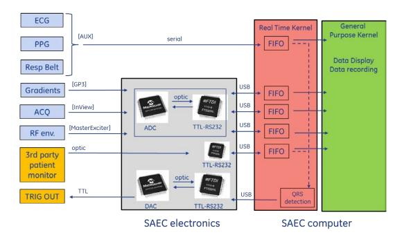
Figure 3.1 – Schematic of the new SAEC system; Blue areas is data provided from MRI system. Indications in [] are the connection ports at the GE HDxt MRI system
