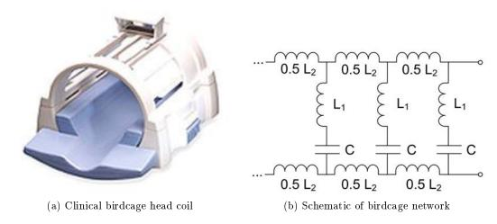
Figure 2.3 – a) Clinical birdcage headcoil, b) Ladder network of a low-pass birdcage coil
