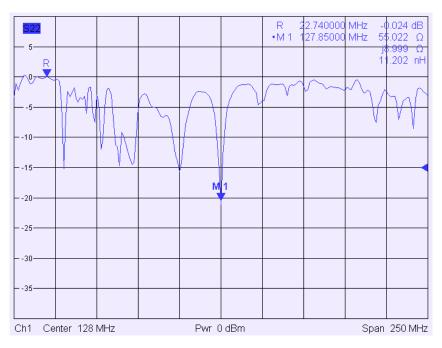
Figure 2.4 – Harmonic frequencies of 3T birdcage body coil; M = Marker at 128MHz Larmon frequency
