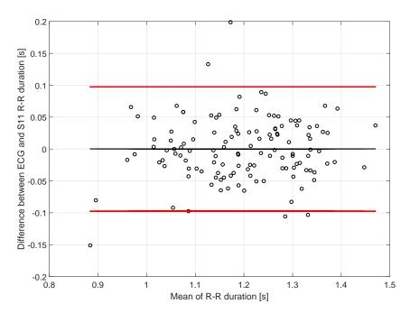
Figure 6.15 – Bland-Altman plot of R-R durations measured from ECG data and S11-data (R<sup>2</sup>=0.86). Red lines indicate  $2\sigma$  standard deviation
