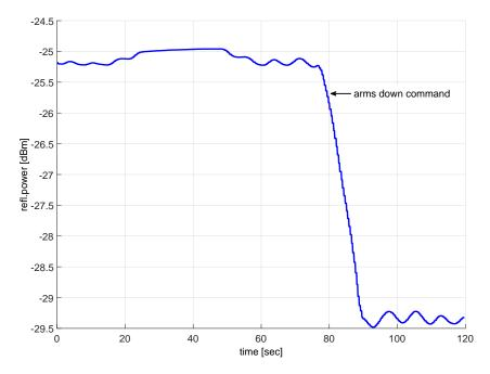
Figure 5.4 – Reflected power level change on arm motion during normal breathing; breathhold between t=25...50 seconds
