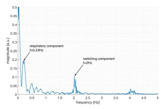
$\label{eq:figure} Figure~5.10-FFT~of~power~signal~of~mode~frequency;~f=0.23Hz~corresponds~to~respiration\\ frequency~of~14cylces/minute;~f=2Hz~reflects~switching~frequency$
