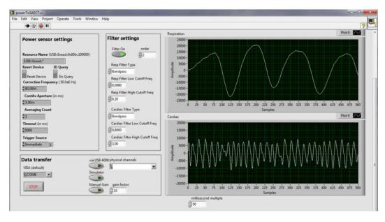
Figure 3.6 – GUI of a LabView application for reflected power measurement. Respiratory and cardiac filtered signal is visualized. Data transfer options, filter parameter and sensor settings are available
