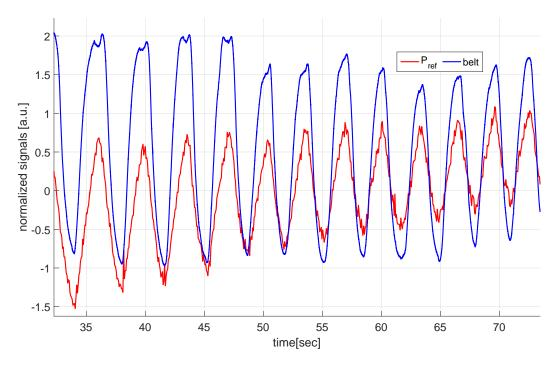
Figure 5.3 – Graphical comparison of reflected power of excitation pulse with respiratory belt
