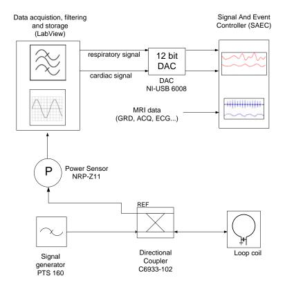
Figure 3.3 – Schematic of motion acquisition by reflected power measurement: A continous wave signal from the signal generator is transferred to the loop coil via a directional coupler. Reflected power is measured at the coupler with a power meter. This power is scaled and filtered and forwarded to a DAC, which converts the signal into voltages for the SAEC input. For comparison physiologic signals and sequence parameters from MRI can be routed to the SAEC
