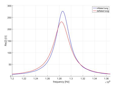
Figure 4.2 – Real value of the simulated coil impedance of deflated (red) and inflated lung (blue). Due to the higher conductivity, the Q-value is lower in the deflated state
