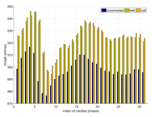
$\begin{array}{c} {\rm Figure~6.12-Image~entropy~over~31~cardiac~phases.~Entropy~of~uncorrected~(blue),~belt} \\ {\rm corrected~(green)~and~S11~corrected~(orange)~of~volunteer~5} \end{array}$
