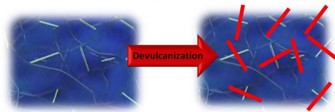
Figure 5: Schematic of devulcanization, where the red blocks represent the breaking of the cross-linkings of the elastomer due to process of devulcanization.
