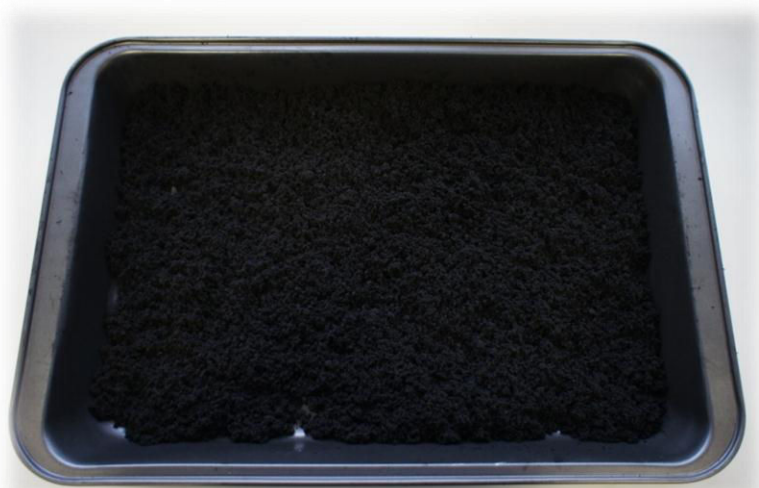
Figure 11: Photo of the GTR5.5 spread in a metallic form to avoid thermal degradation.
