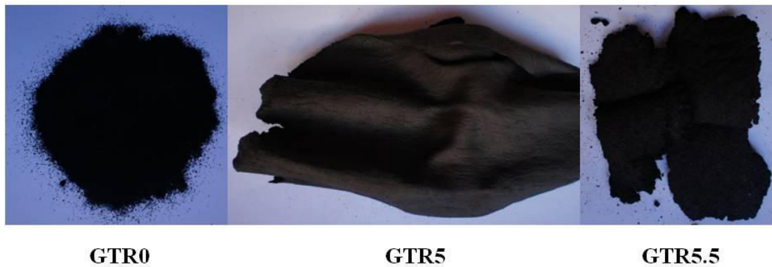
Figure 29: Photos of GTR0, GTR5 and GTR5.5 after remixing in a two roll mill.
