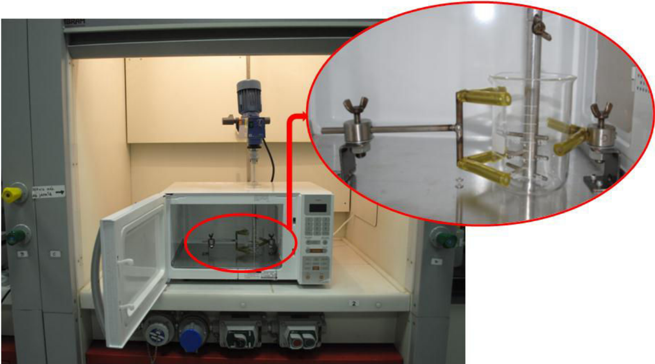
Figure 10: Devulcanization system used, with detail of the stirring rod responsible for rubber mixing during treatment, which prevents its degradation by the action of hot spots (points of high concentration of microwaves due to resonance effects in the cavity of the oven). It can be also observed the clutches system designed to promote good attachment to the container during the process.
