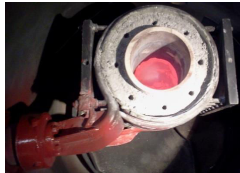
Figure 12: Zoom of the inductor and the crucible inside the vessel (top view)
