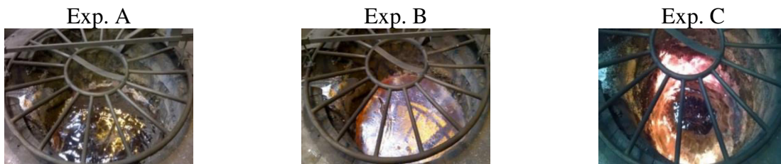
Figure 79: Experimental observations of bath free surface fluctuations during Exp. A, B and C
