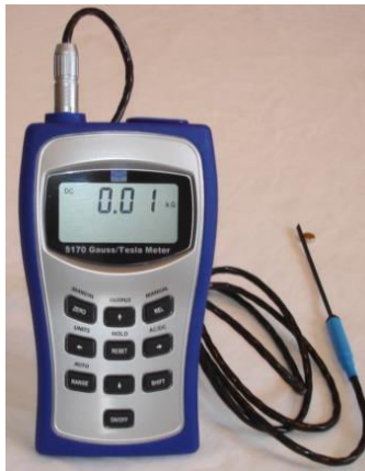
Figure 16: Gaussmeter with axial probe
