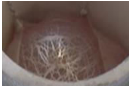
Figure 104: Camera image of oxide layer stretching (Al-7050 at 50 % filling level and P_{\text{gen}} = 15 \text{ kW} )
