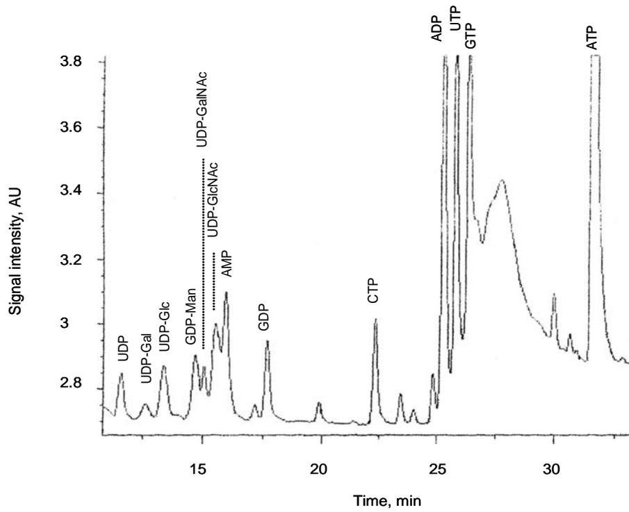
Fig.3: Ion-pair RP-HPLC separation of a 40 $\mu$ l perchloric acid CHO cell extract ( $4 \times 10^6$  cells, 48h-old). Briefly, the cellular pellet was submitted to perchloric acid extraction. After a neutralization step, soluble nucleotides and nucleotide sugars were then analyzed by ion-pair RP-HPLC.
