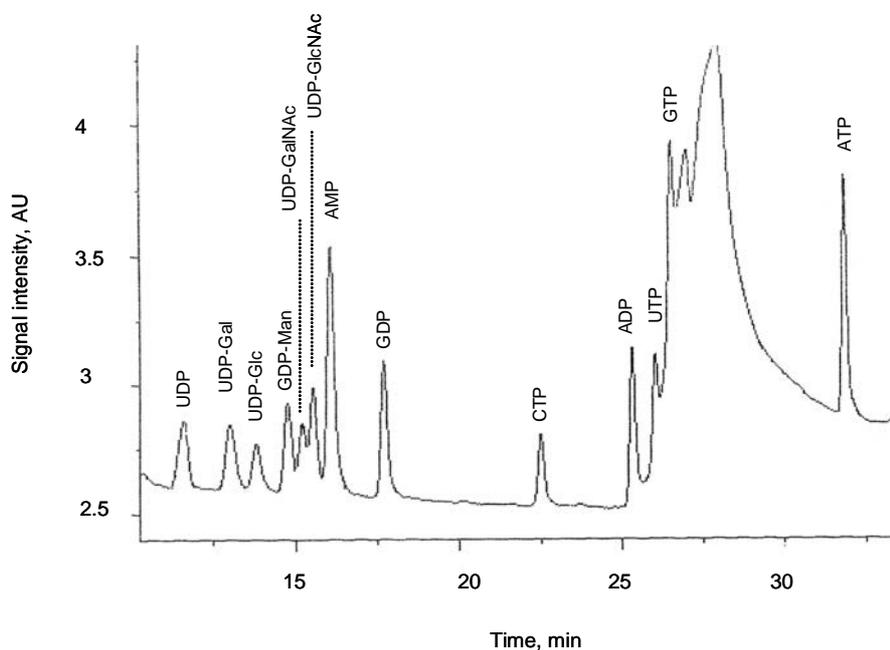
Fig.1: Ion-pair RP-HPLC chromatogram of 30 $\mu$ l of a standard solution of 13 nucleotides and nucleotide sugars. The concentration of each compound was 20 $\mu$ M (600 pmol injected). Separations were performed with a reverse phase column, the wavelength of UV detection was 254 nm, and column temperature was set à 40°C. Details about elution conditions are provided in Materials and Methods.
