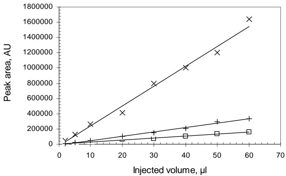
Fig. 4: Linearity between injected volumes and peak areas for perchloric acid cellular extracts ( $4 \times 10^6$  CHO cells, volume injected ranging from 2  $\mu$ L to 60  $\mu$ L). ATP (x), CTP (o), GTP (+), UDP-GlcNAc (◆), GDP-Man ( $\Delta$ ), AMP ( $\square$ ).
