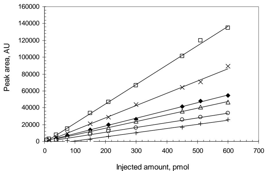
Fig. 2: Calibration curves of standard solution (A) Injected amount ranging from 6000 pmol to 7.5 pmol. (B) Detail, Injected amount ranging from 600 pmol to 7.5 pmol. ATP (×), CTP (○), GTP (+), UDP-GlcNAc (◆), GDP-Man (Δ), AMP (□).
