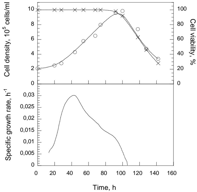
Fig.5: Kinetics of viable cell density (A, ○), viability (A, ×), and specific growth rate (B), during a batch culture of CHO cells.
