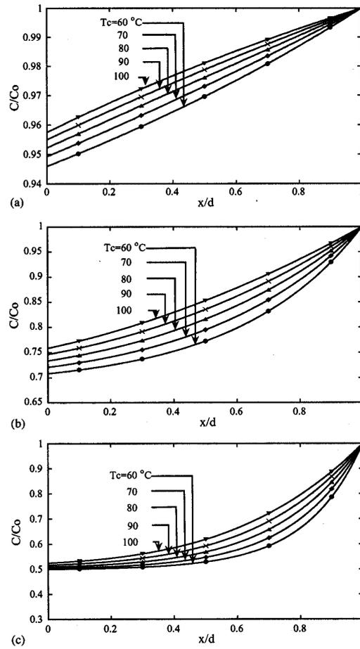
Fig. 7. Effect of  $T_c$  on water concentration distribution with  $T_a = 60^\circ\text{C}$  and constant cathode concentration  $C_c = 1.59 \times 10^{-4} \text{ mol cm}^{-3}$ : (a)  $i = 0.1 \text{ A cm}^{-2}$ ; (b)  $i = 0.5 \text{ A cm}^{-2}$ ; (c)  $i = 1.1 \text{ A cm}^{-2}$ .
