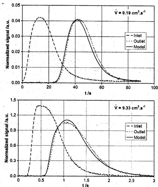
Fig. 4. RTD measurements and modelling of the serpentine flow pattern (signals in arbitrary units).
