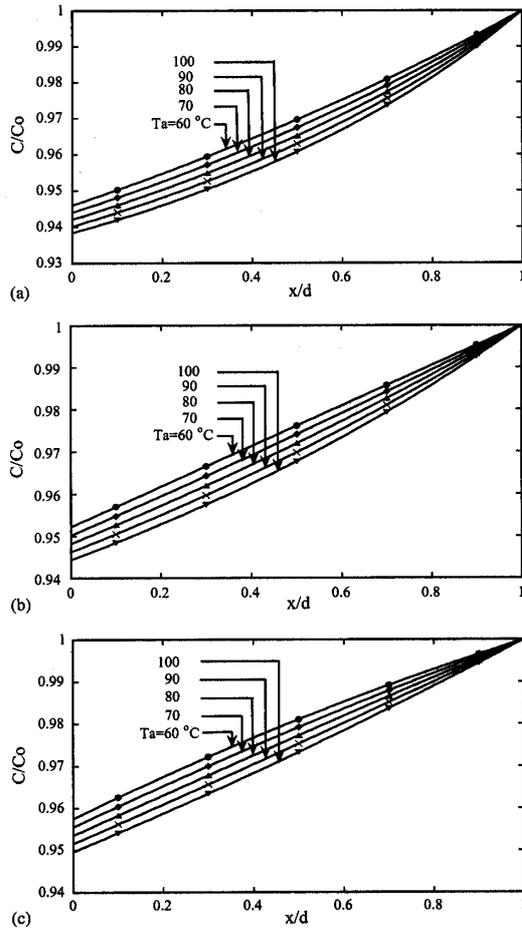
Fig. 6. Effect of  $T_a$  on water concentration distributions with  $i = 0.1 \text{ A cm}^{-2}$  and constant cathode concentration  $C_c = 1.59 \times 10^{-4} \text{ mol cm}^{-3}$ : (a)  $T_c = 60^\circ\text{C}$ ; (b)  $T_c = 80^\circ\text{C}$ ; (c)  $T_c = 100^\circ\text{C}$ .
