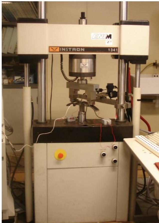
Figure II-14 : Machine de traction/compression INSTRON 1341.
