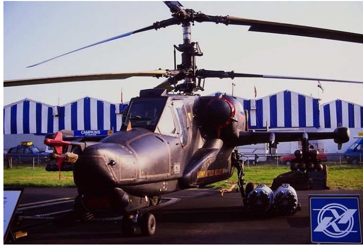
FIGURE 2.8: Hélicoptère bi-rotor coaxial
