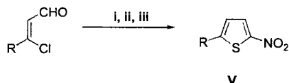
Scheme 2. Substituted 2-nitrothiophenes synthesized by our team. (i) \text{Na}_2\text{S}\cdot 9\text{H}_2\text{O} , DMF; (ii) \text{BrCH}_2\text{NO}_2 ; (iii) NaOH.
