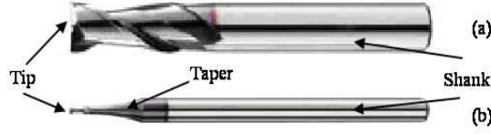
Figure 5.1: Geometric comparison between (a) macro mill and (b) micromill
