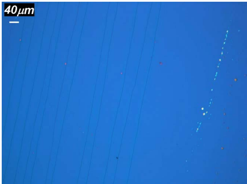
Fig. 73: Image of the surface of the sample A after the annealing obtained with an optical microscope (X100). The black lines are cracks.
