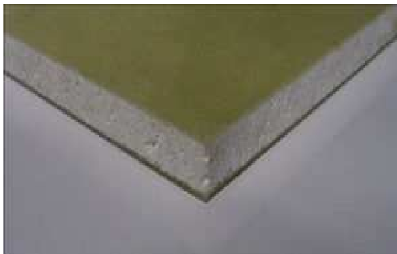
Figure 2.1 Structure sandwich en YmaCell
