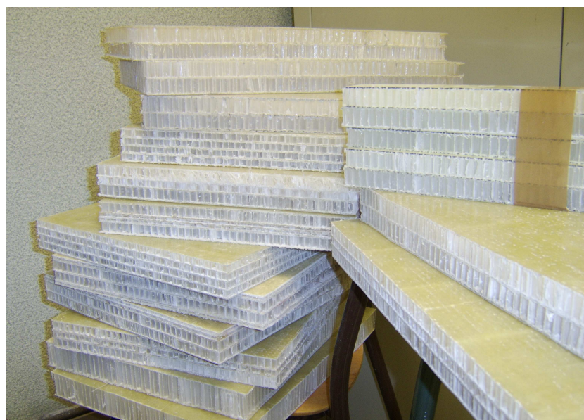
Figure 2.4 Structure sandwich multicouches
