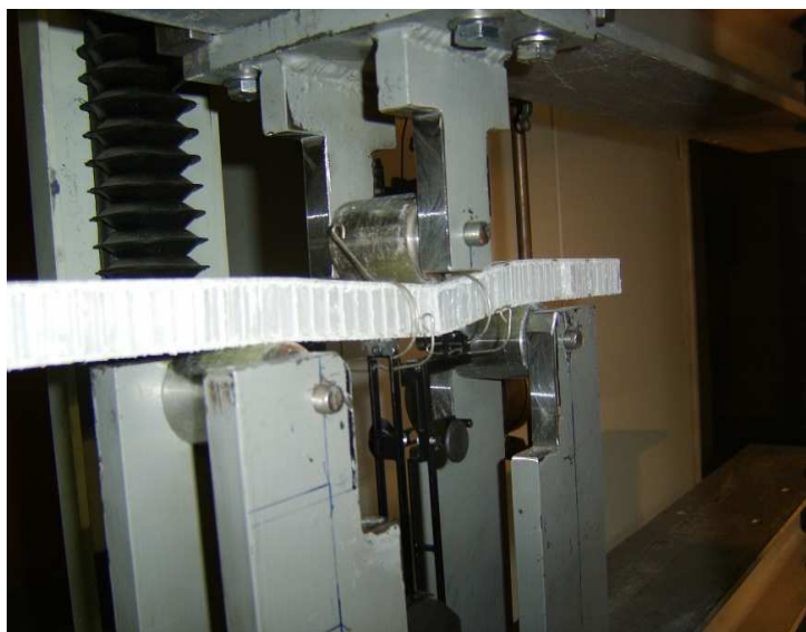
Figure 2.12 Essai de flexion 3-points
