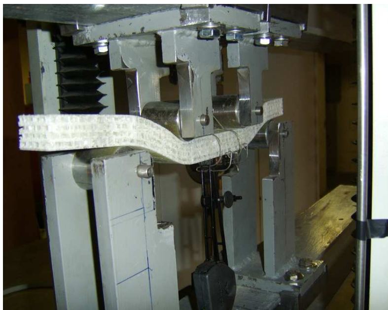
Figure 2.11 Essai de flexion 4 points
