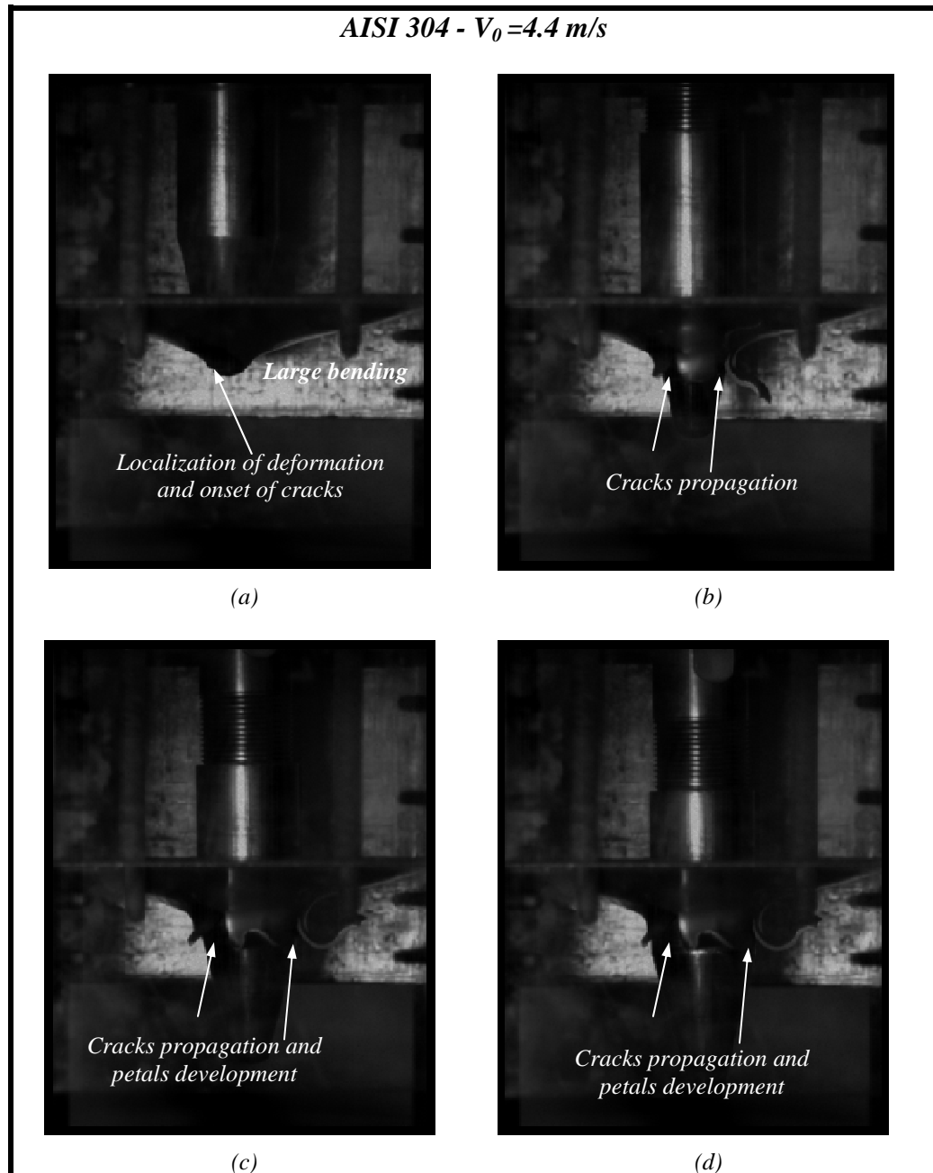
Fig. 5.34. Different stages of the perforation process for V_0 = 4.4 \text{ m/s} at room temperature. (a) Localization of deformation and onset of cracks. (b) Cracks progression and generation of petals. (c) Development of petalling. (d) Complete passage of the impactor and petalling failure mode.
