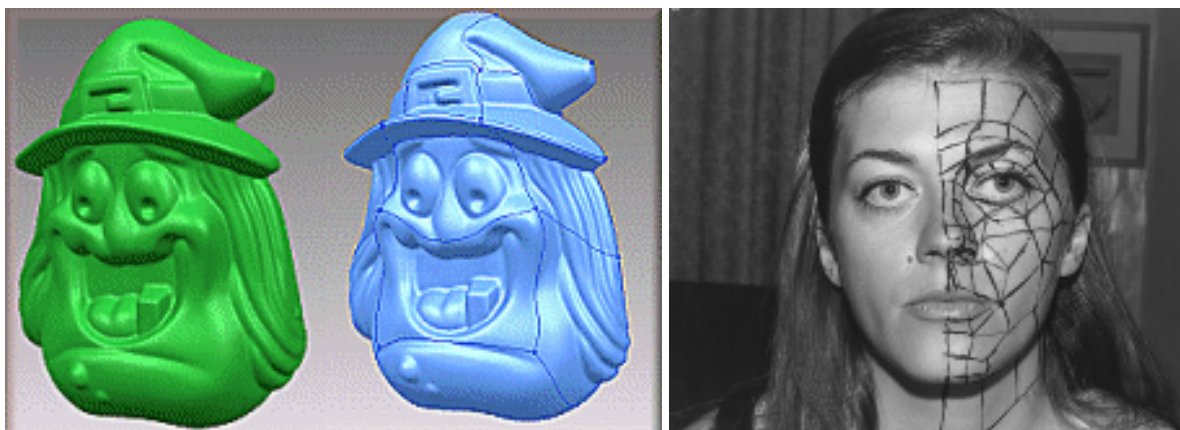
FIG. F.2: Left : manual design of a CAGD/CAM control mesh [Rap] from a triangular mesh ; Right : digitization of a real object by manual acquisition (the image is taken from Gouraud's thesis [Gou71b]).
