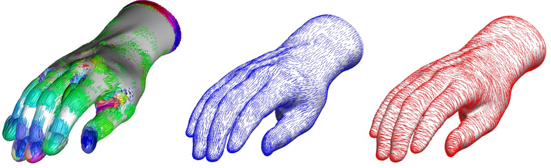
FIG. D.4: Left : Curvature tensor visualized as ellipsoids ; center (resp. right) : principal direction field corresponds to the minimum (resp. maximum) curvature.
